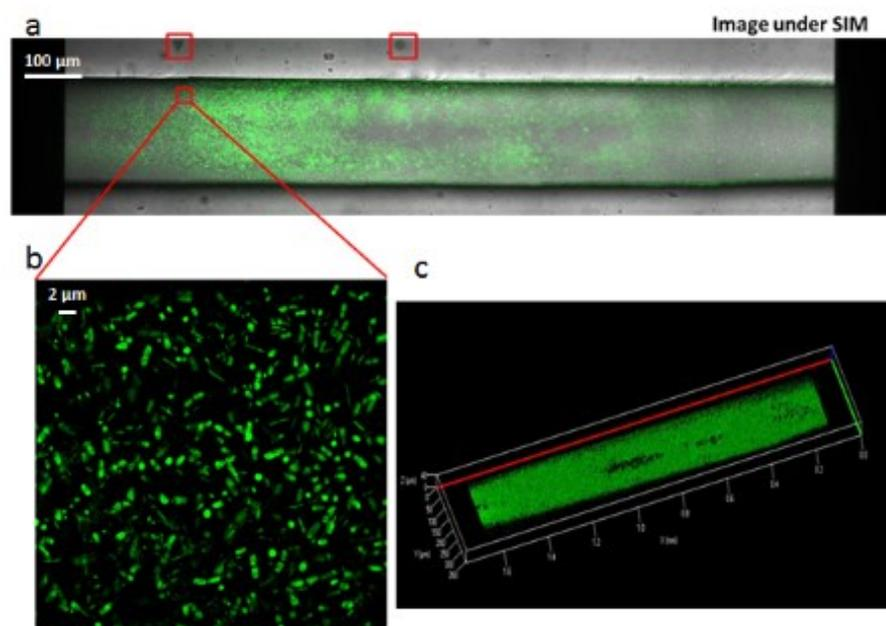
**Fig S1a.** SIM images of (a) the microfluidic channel; (b) the zoomed-in area in the red square in a; and (c) a view of the channel reconstructed using ImageJ software.
