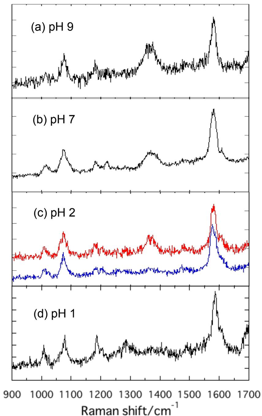
**Fig. S1** SEHRS spectra from the optically trapped AgNPs adsorbed with p-MBA on the conventional glass slide in the suspension at pH (a) 9, (b) 7, (c) 2, (d) 1 by addition of (a) 0.01 M  $\text{Na}_2\text{B}_4\text{O}_7$ , (b) 0.02 M NaCl aqueous solution without and (c, d) with  $\text{H}_2\text{SO}_4$  to the Ag colloidal suspension in a ratio of 1:3 (v/v).
