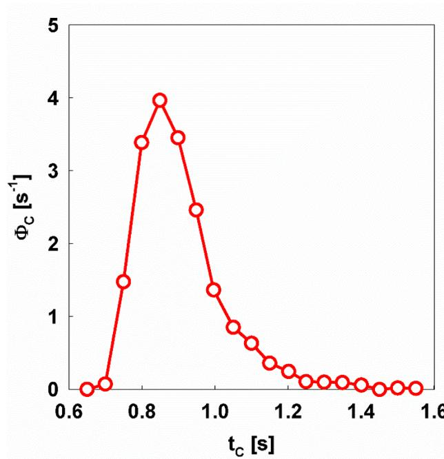
**Figure S3:** Response time distribution function of the TSI WCPC Model 3786, reported in Oberreit et al (2014)<sup>2</sup>. The distribution peak value is  $t_C = 0.846$  s.
