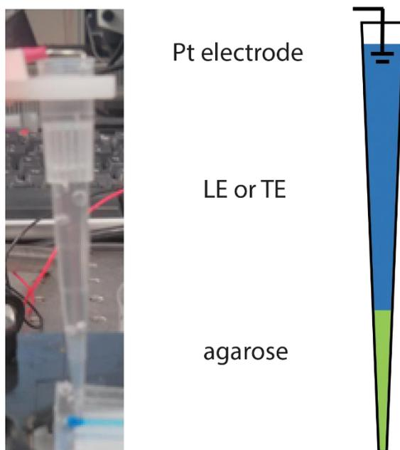
**Figure S3.** Buffering reservoir design consisting of a 1 mL pipette tip filled with LE or TE buffer, and solidified agarose on the bottom to prevent leakage. A platinum wire electrode is connected to an external voltage source. This reservoir design allows sufficient buffering capacity and prevents bubbles from entering the channel.
