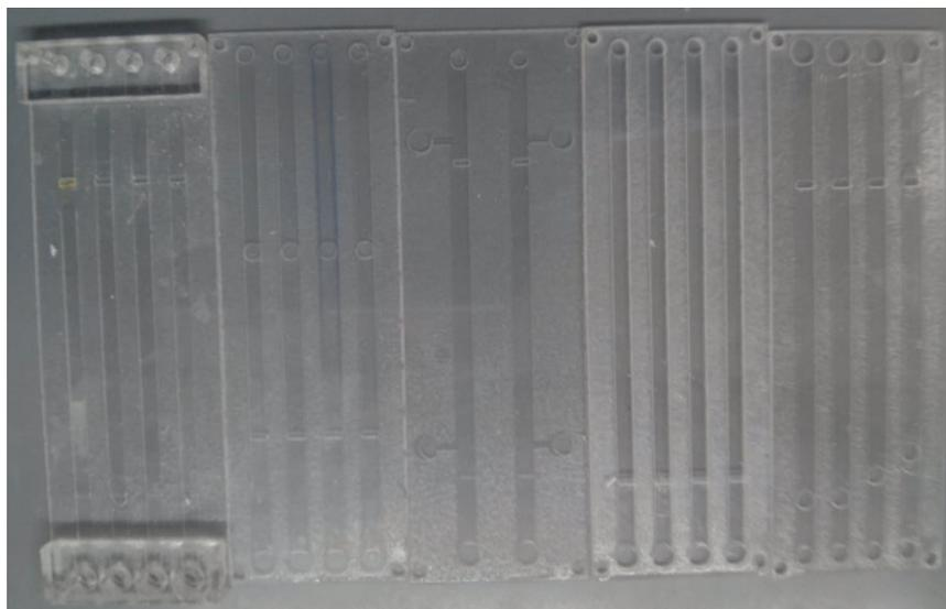
**Figure S2.** Select device designs generated with rapid prototyping approach. During the development of this assay, we explored different device designs and geometries to optimize ITP preconcentration and fractionation. Our rapid-prototyping approach involved using AutoCAD software to design, and a CO<sub>2</sub> laser cutter to generate microfluidic channel geometries in PMMA sheets. This approach allowed to test several designs with minimal turnaround time.
