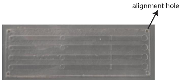
**Figure S1.** Schematic of completed device highlighting the alignment holes at each edge.
