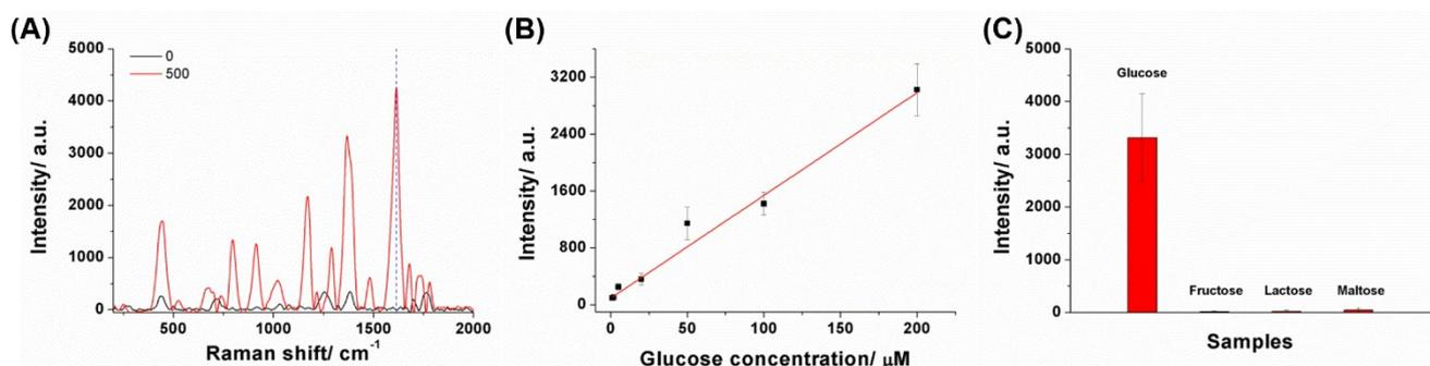
**Figure S4.** (A) SERS spectra in the absence and presence of 500 μM glucose. (B) Linear response of SERS signal of MG at 1615 cm<sup>-1</sup> versus glucose concentration. (C) Selective detection of glucose against other saccharides (such as fructose, lactose and maltose). Error bars indicate standard deviations of three independent measurements.
