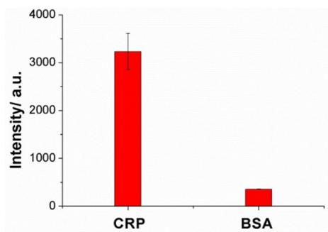
**Figure S5.** Raman intensity of MG at 1615 cm<sup>-1</sup> versus 1000 ng/mL CRP and 10 mg/mL BSA. Error bars indicate standard deviations of three independent measurements.
