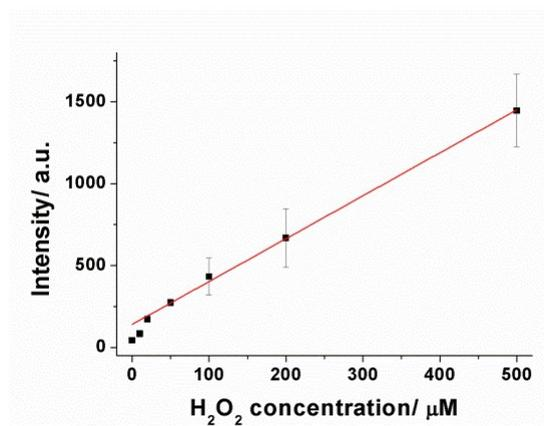
**Figure S3.** Linear response of SERS signal of MG at  $1615\text{ cm}^{-1}$  versus  $\text{H}_2\text{O}_2$  concentration. Error bars indicate standard deviations of three independent measurements.
