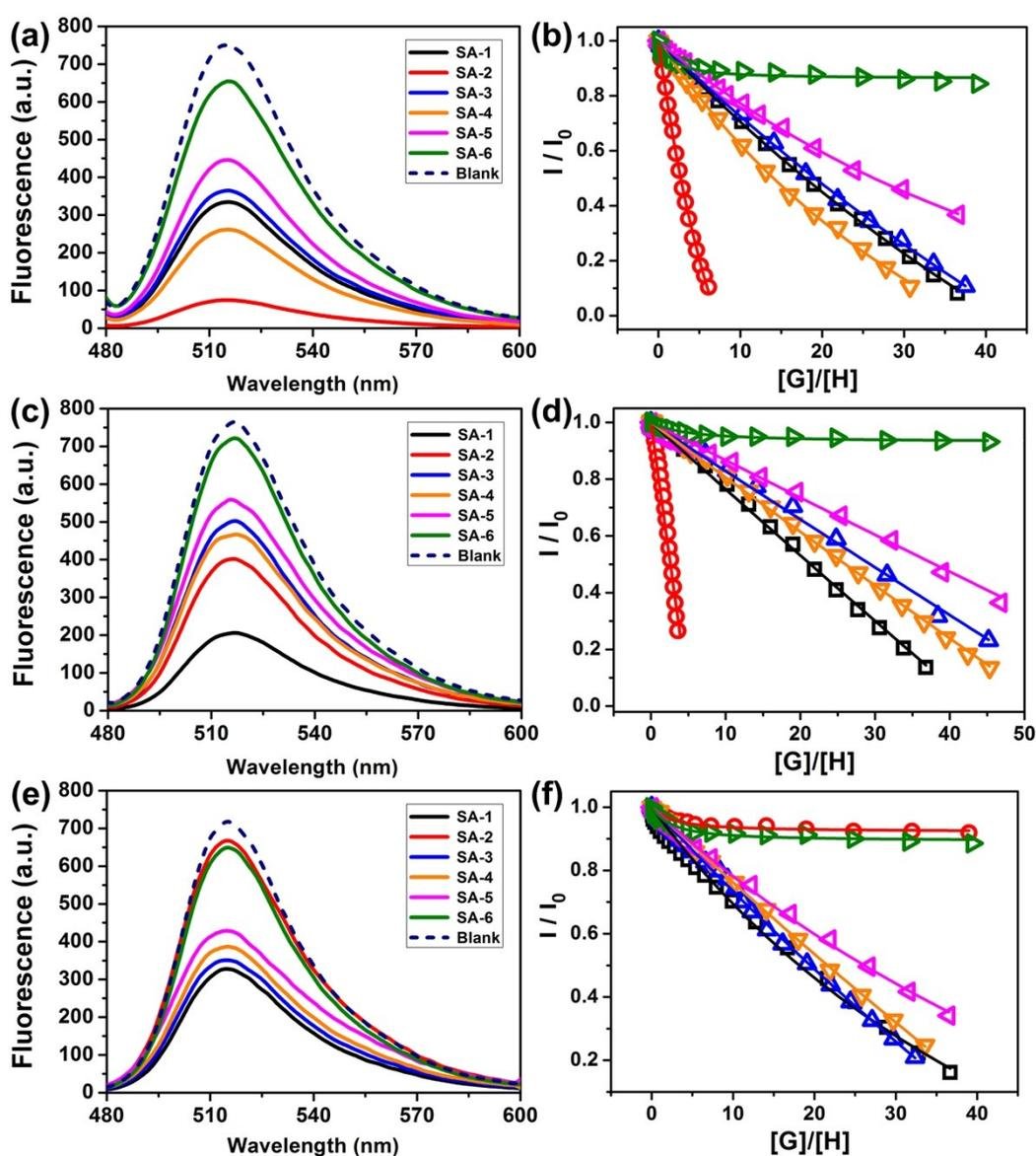
**Fig. S2** Fluorescence spectra ( $\lambda_{ex}$ : 470 nm) of FL-DP (a), FL-DA (c) and FL-DD (e) solutions (6  $\mu$ M) upon the addition of 20 equivalents of SA derivatives in Tris-buffer solution (1 mM, pH 7.4) at 20 °C, and corresponding dynamic fluorescent intensity ( $\lambda_{em}$ : 514 nm) changes of FL-DP (b), FL-DA (d) and FL-DD (f) solutions with the addition of various equivalents of different SA derivatives in Tris-buffer solution (1 mM, pH 7.4) at 20 °C.
