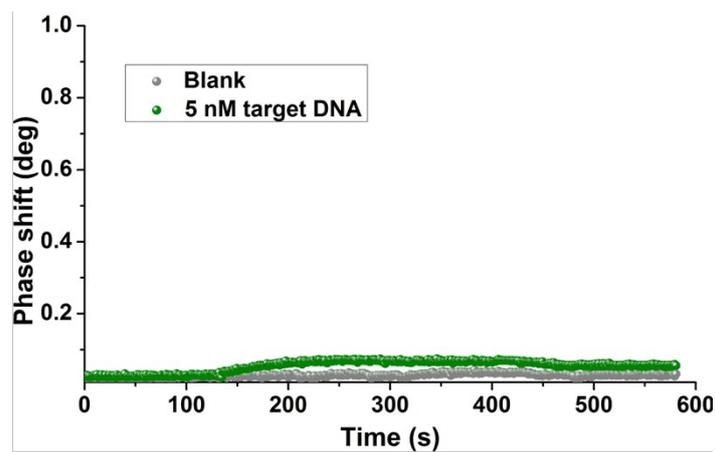
**Figure S4.** The phase shift of the SAW sensor in response to 5 nM target DNA without signal amplification
