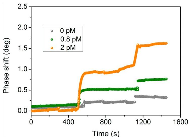
**Figure S3.** The phase shift of the Love-SAW sensor in response to different concentrations of target DNA with synergic signal amplification. The detection limit of 0.8 pM is detectable.
