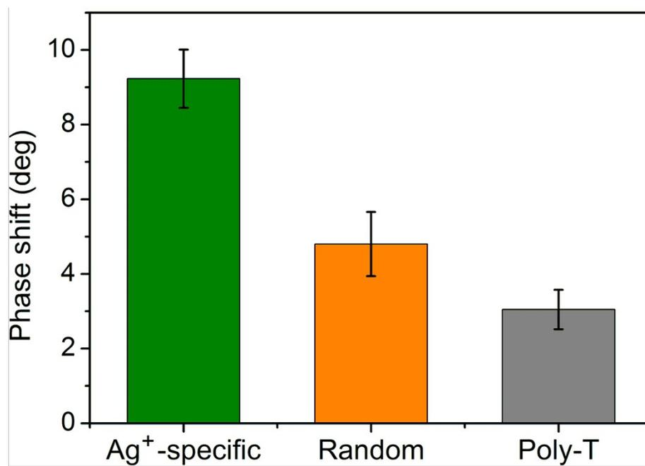
**Figure S1.** The Love-SAW phase shift of using of different sequences (Ag<sup>+</sup>-specific probe, random sequence and poly-T in Table 1) in the presence of 0.5 nM target DNA with synergic signal amplification.
