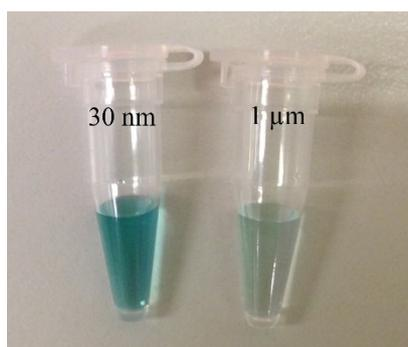
**Fig. S1.** Nanozyme activities of 30 nm and 1 μm magnetic nanoparticles, respectively.
