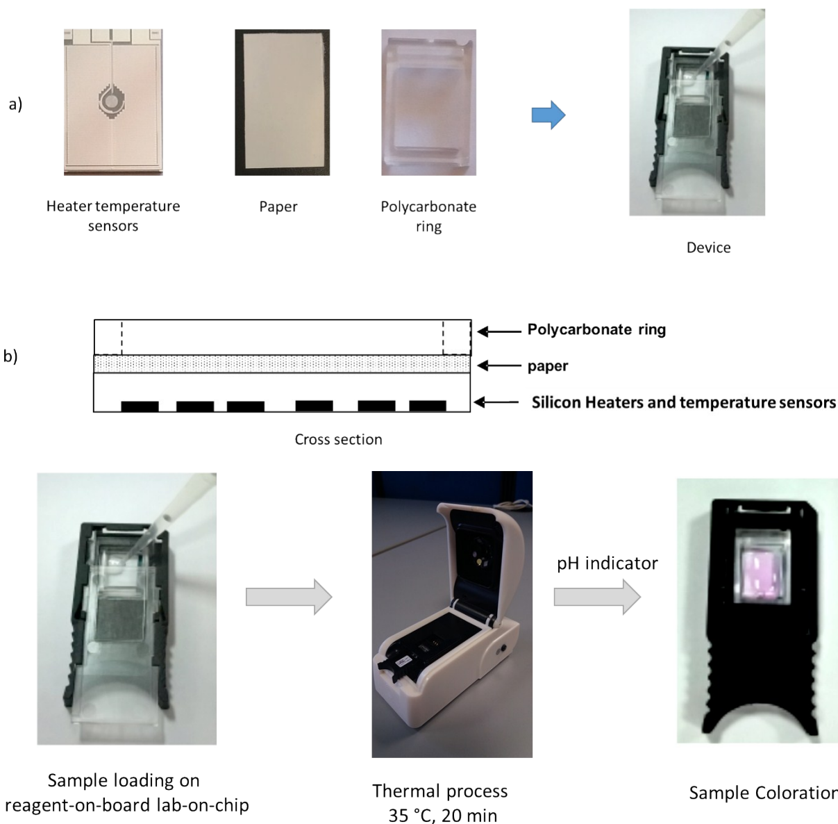
Fig. SI1 Paper-based Lab-on-Chip: a) components and b) cross section and c) full process on lab-on-chip
