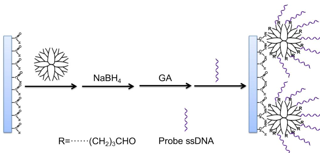
**Fig. S1.** Fabrication process of 3D DNA microarray.
