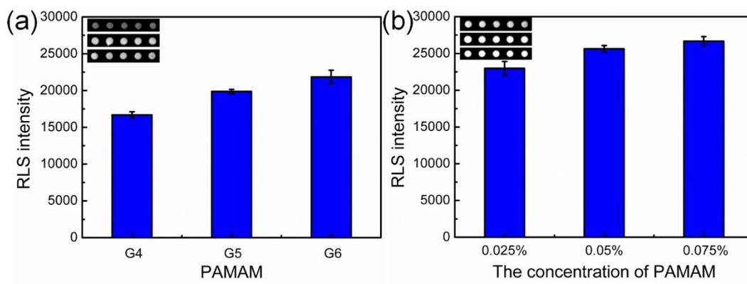
**Fig. S2.** RLS images (inset) and corresponding RLS intensities of 3D DNA microarrays fabricated on different kinds of dendrimer (0.025 % (w/w) PAMAM G4, G5, G6) (a) and different concentrations of PAMAM G6 dendrimer (b) modified slides. 300 pM ssDNAs<sub>i</sub>@GNPs were hybridized with immobilized Pi on 3D DNA microarray at 42 °C. The concentration of Pi in printing solution is 0.5 μM.
