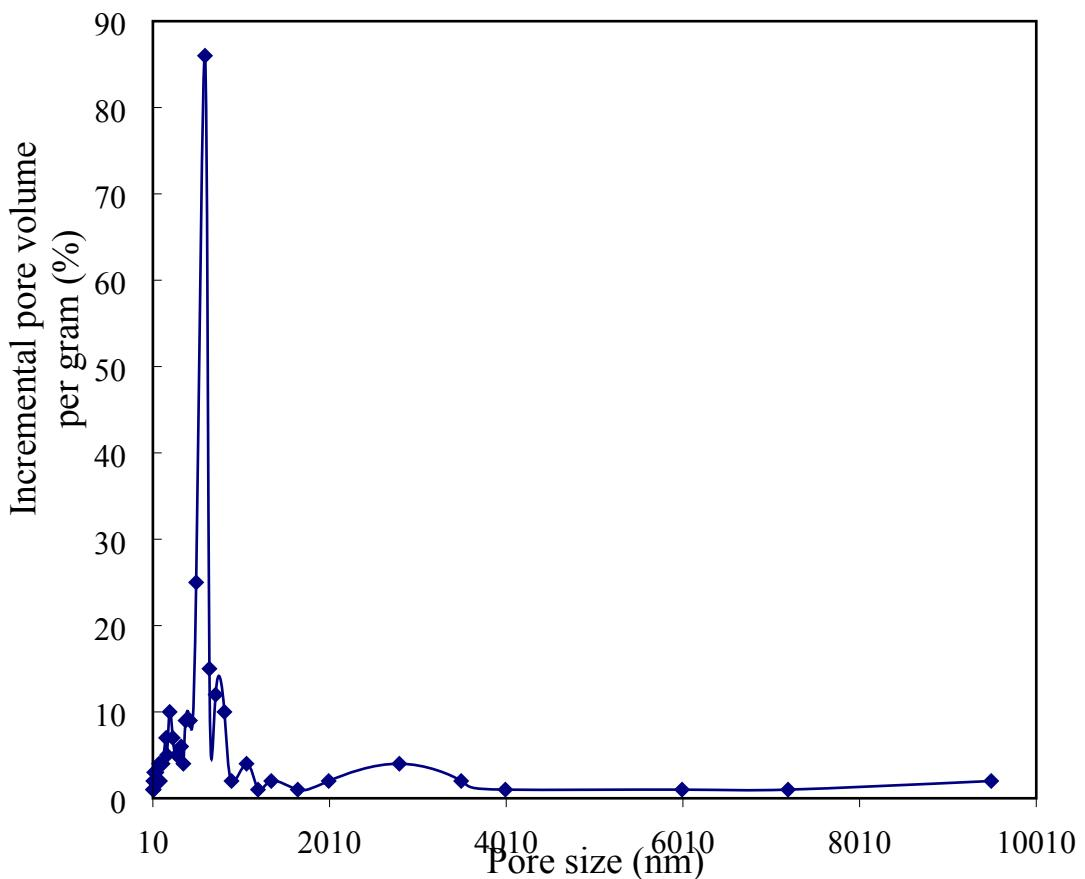
**Fig.S3.** The PSD plot of PIL/MIP
