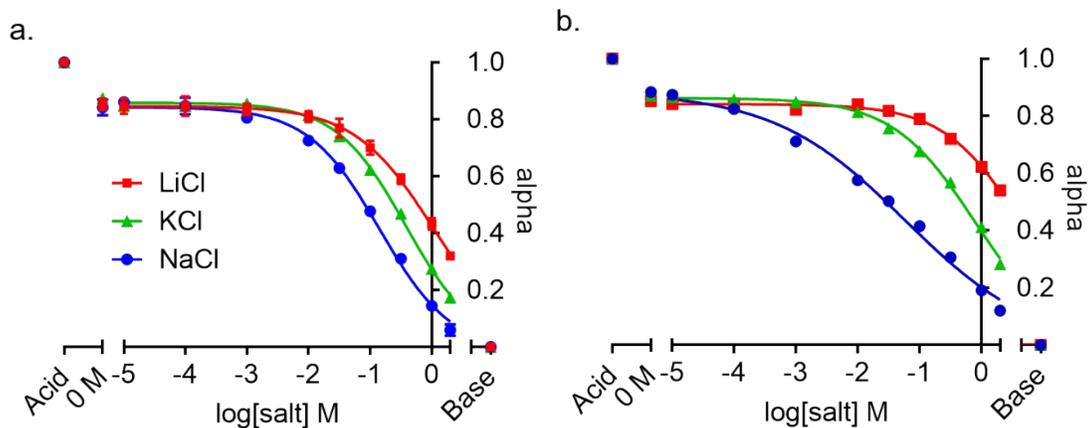
**Figure S-2.** (a) Normalized fluorescence response of Blueberry-CD nanosensors to either NaCl, KCl, or LiCl. (b) Normalized response of traditional chromoionophore-ionophore Na-nanosensors to NaCl, KCl, or LiCl. The Blueberry-CD nanosensors demonstrate selectivity against  $K^+$  and  $Li^+$  that is in agreement with that of the traditional chromoionophore-based nanosensors. Error bars represent SD ( $n = 5$ ) and are not shown if smaller than the symbol height.
