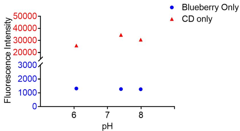
**Figure S-3.** CD-free nanosensors and the Blueberry dye-free nanosensors showed stable fluorescence at an emission of 480 nm (excitation 420 nm) for the biological pH range of pH 6, pH 7, and pH 8. Error bars represent SD (n=3) and are not shown if smaller than the symbol height.
