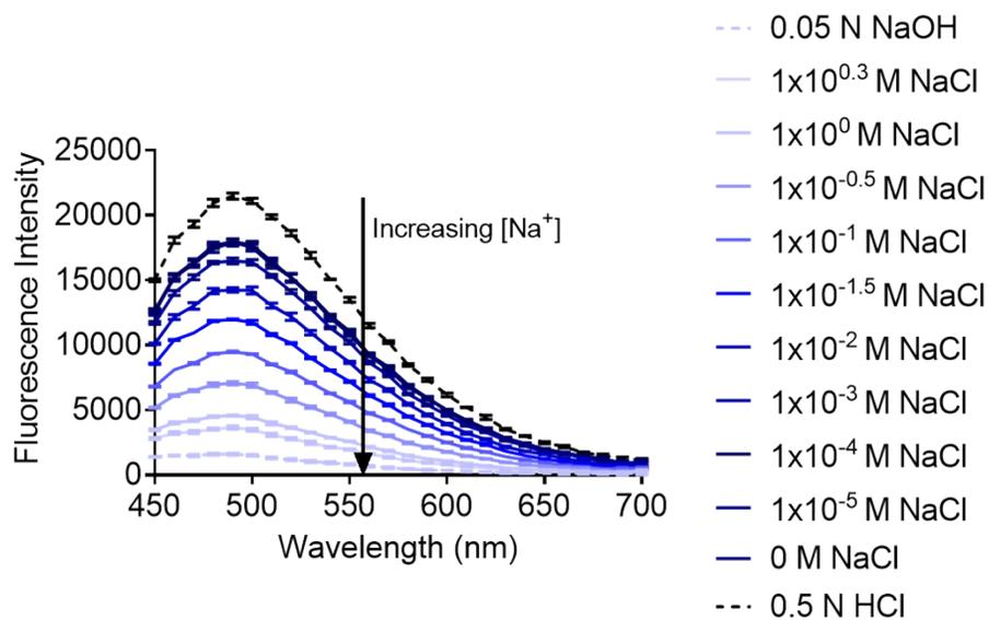
**Figure S-1.** Labeled plot of **Fig. 4** in main text. Emission spectra of Blueberry-CD nanosensors at 420 nm excitation in 0.05 N NaOH, 0.50 N HCl, and a range of NaCl concentrations in buffered HEPES/TRIS (pH 7.4). Error bars represent SD (n = 3).
