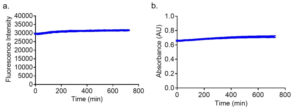
**Figure S-5.** a) Fluorescence intensity of Blueberry-CD nanosensors and (b) Absorbance of Blueberry-CD nanosensors observed every 30 s for 720 min, demonstrating no detectable changes in optical properties, respectively. Error bars ( $n = 5$ ) are shown and are represented by the line width.
