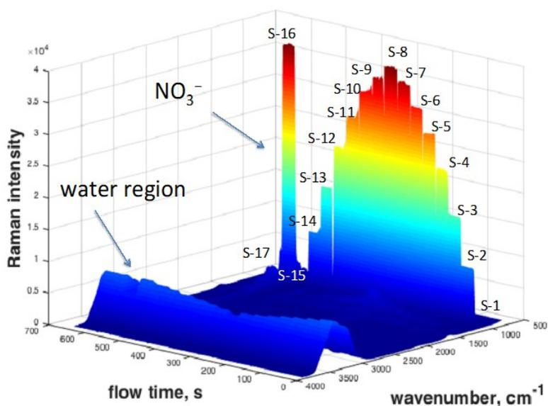
**Figure SI-2:** The sequence of Raman spectra recorded by the micro-Raman probe as a function of time for a series of  $\text{HNO}_3$  solutions passed through a 70  $\mu\text{L}$  flow cell (aperture diameter 3 mm). The 648 spectra recorded during the flow run are presented sequentially along the flow time axis in the order they were recorded. The spectra were recorded over a spectral range of 750  $\text{cm}^{-1}$  to about 4000  $\text{cm}^{-1}$ .
