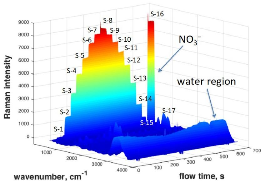
**Figure SI-3:** The sequence of Raman spectra recorded by the micro-Raman probe as a function of time for a series of  $\text{HNO}_3$  solutions passed through an 8  $\mu\text{L}$  flow cell (aperture diameter 3 mm). The 648 spectra recorded during the flow run are presented sequentially along the flow time axis in the order they were recorded. The spectra were recorded over a spectral range of 750  $\text{cm}^{-1}$  to about 4000  $\text{cm}^{-1}$ .
