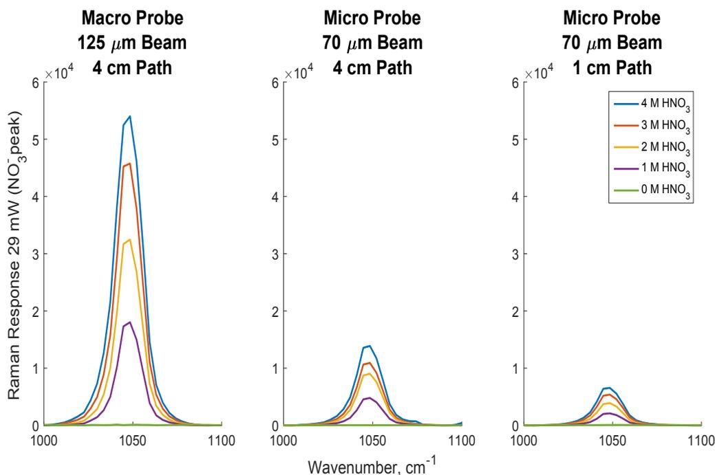
**Figure SI-1:** Comparison of Raman spectra collected on the 125  $\mu\text{m}$  macro probe and the 70  $\mu\text{m}$  micro probe. A 4 cm path length was available for samples recorded using 2 dram glass vials, while the path length was reduced to 1 cm for samples recorded in the 8  $\mu\text{L}$  flow cell.
