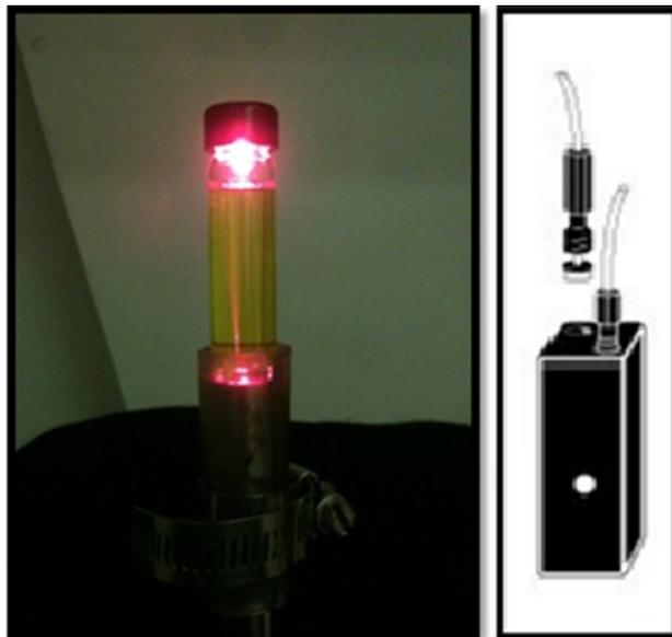
**Figure SI-4. Left** – Glass vial (2 dram) containing a solution sample positioned above the Raman probe using a plastic collar to secure the sample. **Right**—Schematic diagram of a Starna™ 585.3-Q-10-Z15 micro flow cell showing aperture and ports for solution flow through.
