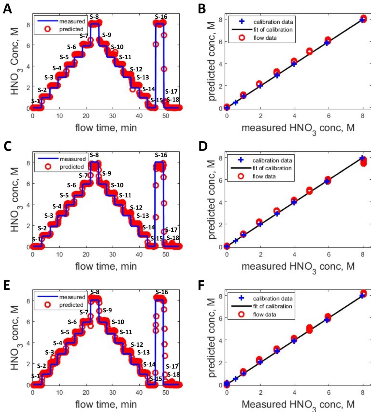
**Figure SI-5:** (A) PLS model results and (B) model fit for the macro Raman probe paired with the 70  $\mu\text{L}$  flow cell; (C) PLS model results and (D) model fit for the macro Raman probe paired with the 8  $\mu\text{L}$  flow cell; (E) PLS model results and (F) model fit for the micro Raman probe with the 8  $\mu\text{L}$  flow cell.
