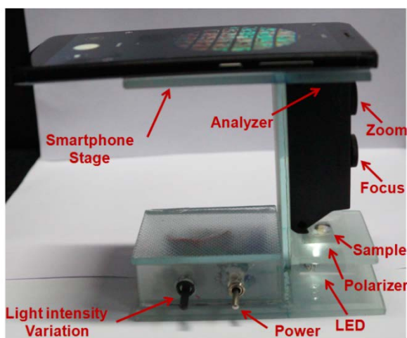
Fig. S1. Photograph of the smartphone based sensing device made by glass.
