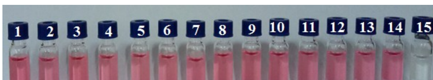
Fig. S7 The color change of probe Mi (5 \mu\text{M} ) in presence of various analytes including: 1.none, 2. \text{SCN}^- , 3. \text{NO}_2^- , 4. \text{SO}_4^{2-} , 5. \text{S}_2\text{O}_3^{2-} , 6. \text{ClO}^- , 7. \text{H}_2\text{O}_2 , 8. \text{F}^- , 9. \text{Cl}^- , 10.Cys, 11.Hcy, 12.GSH, 13. Citric acid, 14.Gly, 15. \text{HS}^- (20 equiv of 2-14, 10 equiv of 15). ( \lambda_{\text{ex}}/\lambda_{\text{em}} = 520/596 nm. slits: 5 nm/10 nm)
