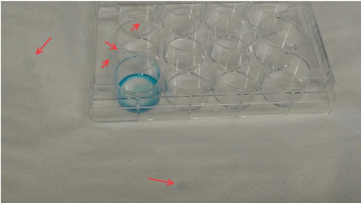
**Figure SI-4:** Spills during processing of a well. The red arrows show zones where spills had been detected after scraping of the well.
