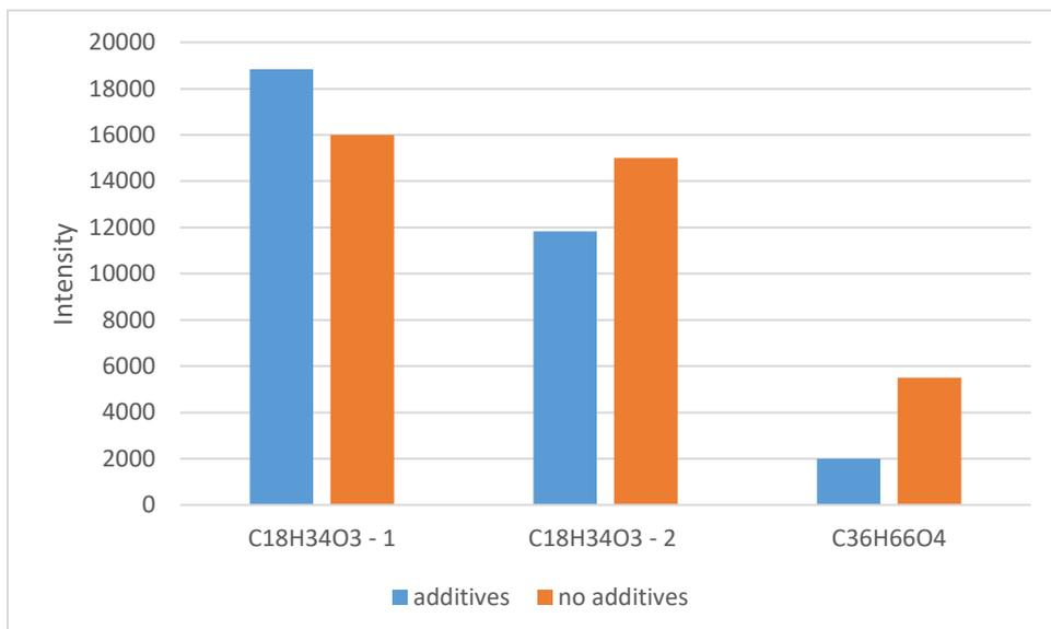
**Figure SI-5:** Degradation products of Oleic acid when the samples were processed with and without additives.
