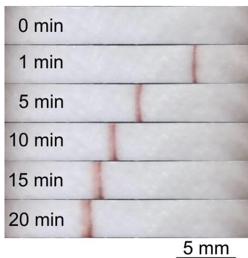
Fig. S5 Images of the stacking band of BHB at different time points. The band was still on the paper channel with sight dispersion even the stacking lasted 20 min.
