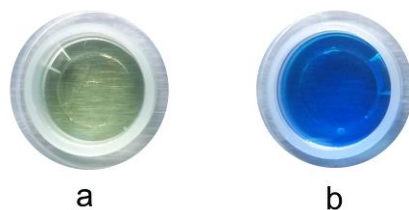
Fig. S3 pH change in the cathode sample reservoir. (a) For deionized water, it is bluish green in the presence of the acid-base indicator, bromothymol blue (BTB). (b) After an electric connection for 180 s, with the addition of BTB, the color changes to blue in response to the increase in pH caused by water electrolysis. Note that the active indication range of BTB is from a pH of 6.0 (yellow) and 7.6 (blue), while it is bluish green in neutral solution. BGE was 100 mM \text{NH}_4\text{Cl} . Other experimental parameters were the same as in Fig. S1.
