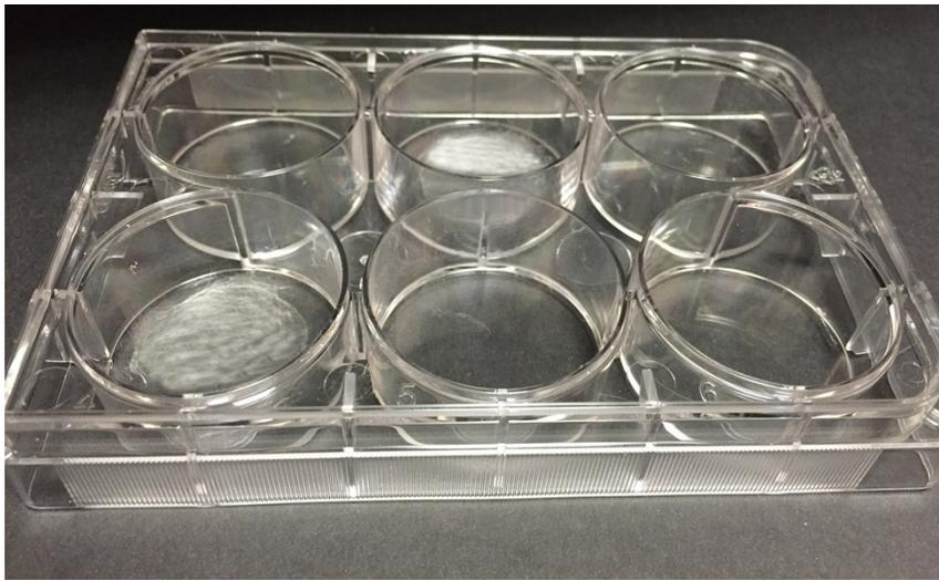
Figure S8. Wind-spun fiber deposition in a 6-well plate for 3D cell culture. PCL (12%) fibers were coated in wells B1 and A2 in the plate at 10 psi sheath N<sub>2</sub> pressure.
