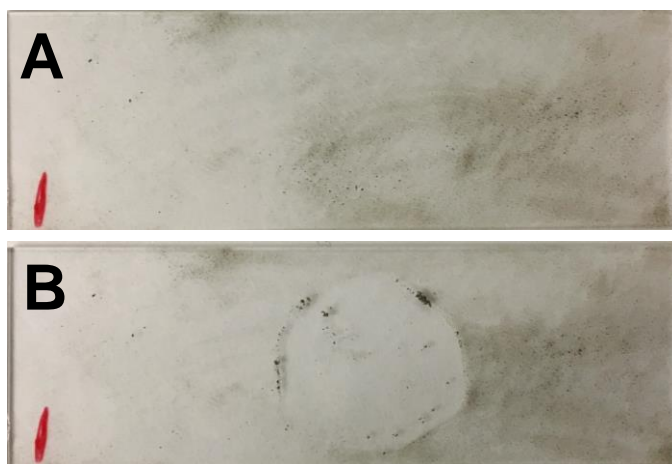
Figure S-2. Photos of a glass slide coated with a layer of latent fingerprints and soil (A) prior to surface swabbing via PSI and (B) after swabbing for the purpose of screening illicit drug residues
