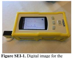
Tactic ID with a 90° sampling accessory, which is placed to focus the laser light on the center of the membrane address.
