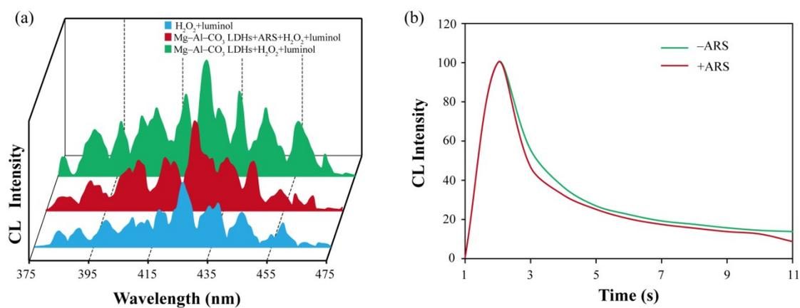
**Fig. S3.** (a) CL spectra of  $\text{H}_2\text{O}_2$ -luminol system without or with addition of Mg-Al- $\text{CO}_3$  LDHs or Mg-Al- $\text{CO}_3$  LDHs + ARS. (b) CL kinetics of LDH- $\text{H}_2\text{O}_2$ -luminol system in the absence (green line) and presence of ARS (red line).
