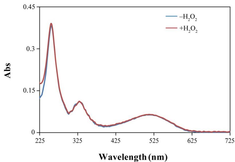
**Fig. S4.** UV-Vis absorption spectra of ARS solution (20 μM) in the absence (blue line) and presence (red line) of 750 μM H<sub>2</sub>O<sub>2</sub>.
