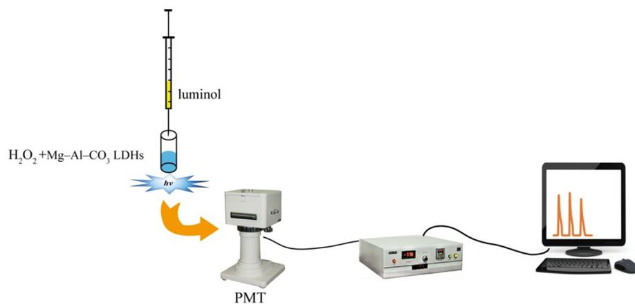
**Fig. S1.** Schematic diagram of CL detection coupled with static injection system.
