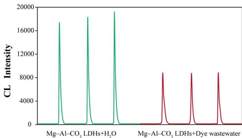
**Fig. S8.** CL signals of LDH-H<sub>2</sub>O<sub>2</sub>-luminol system without (green line) and with (orange line) the addition of dye wastewater.
