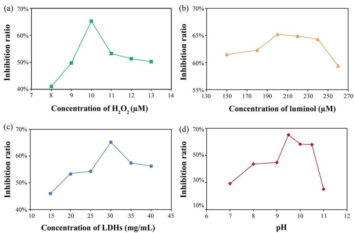
**Fig. S6.** CL inhibition ratio caused by ARS under different  $H_2O_2$  concentration (a), luminol concentration (b), LDHs concentration (c) and pH (d).
