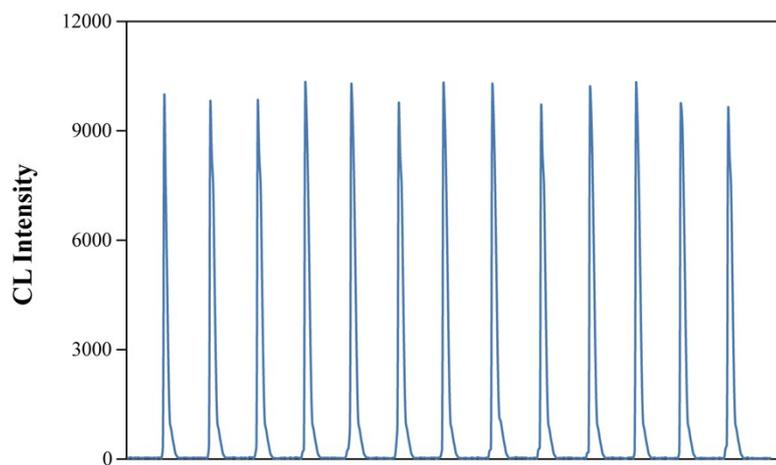
**Fig. S7.** CL signals of LDH-H<sub>2</sub>O<sub>2</sub>-luminol system for 13 repeated measurements in the presence of ARS (1 μM).
