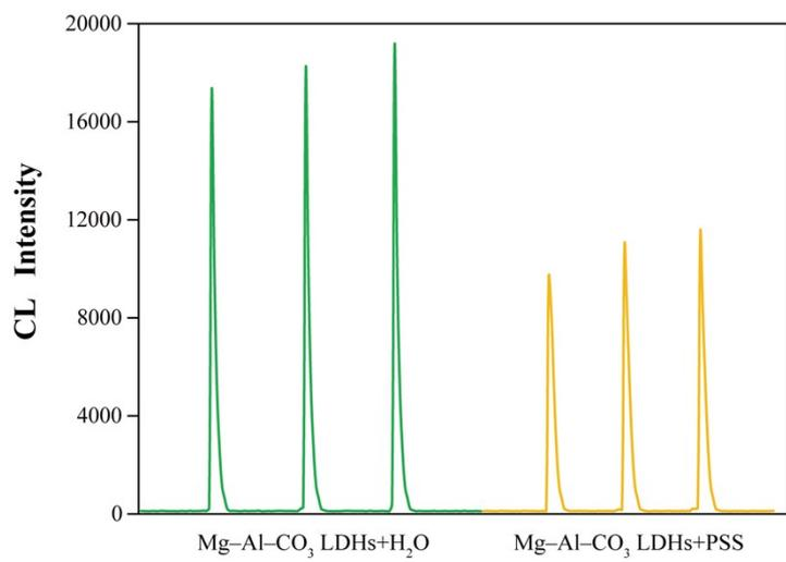
**Fig. S5.** CL signals of the H<sub>2</sub>O<sub>2</sub>-luminol system in the absence and presence of PSS (sulfonic group concentration, 120 μM).
