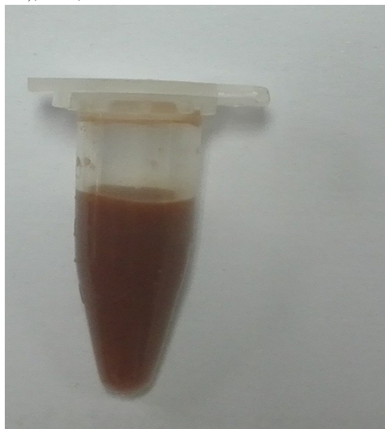
Figure. S-4. Photographic images of \text{Fe}_3\text{O}_4@\text{PMAA}@\text{PEI} dispersing in \text{NH}_4\text{HCO}_3 buffer solution (pH=8.0)
