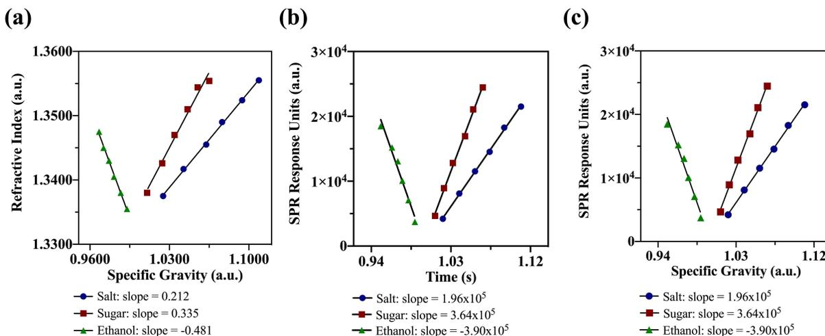
Figure S1: Correlation of RI values (acquired by ATAGO refractometer) and SG values (acquired by Anton Paar density/specific gravity meter) for various aqueous samples.
