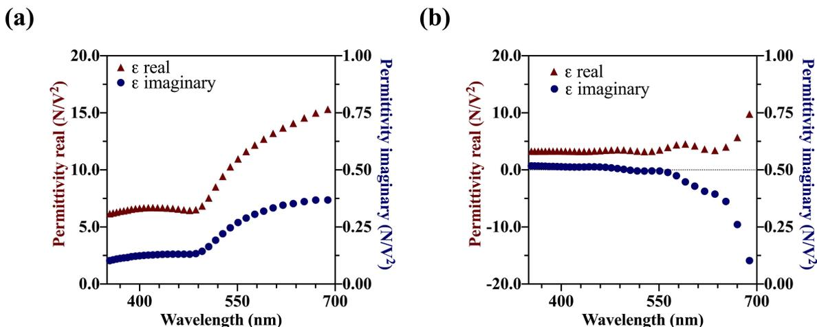
Figure S2: Real and imaginary parts of permittivity of the (a) Au SPR and (b) Au-GO SPR chip surfaces.
