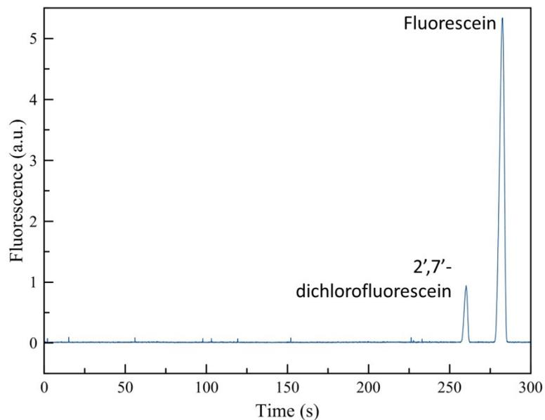
Electropherogram of fluorescence detection of fluorescein and 2',7'-dichlorofluorescein. Analytes were separated in boric acid buffer (pH=9.2) with a field strength of 330 V/cm. For a 1.0 nL injection up to 65,900 plates and 39,800 plates were achieved for 2',7'-dichlorofluorescein and fluorescein, respectively.
