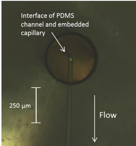
Micrograph of the PDMS channel sealed on to the end of the capillary. The channel is sealed so that the edge of the channel lines with the edge of the inner diameter of the capillary to avoid any dead volume.
