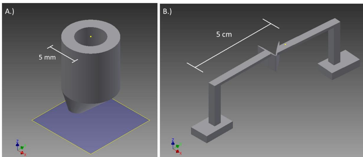
Schematics of the A.) syringe attachment for unclogging the capillary loop and B.) the clip for applying pressure onto the PDMS microchip to prevent delamination. The parts were designed with AutoDesk Inventor 2015 software and printed with Stratasys MOJO Desktop 3D printer. The syringe attachment is adhered to a vacuum luer with a vacuum cup attached before use with a syringe. When put together, the device is used to clean the capillary and prep it before use at the beginning of each day.
