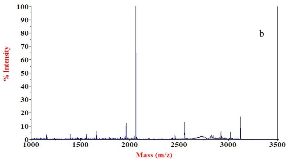
**Fig. S6** MALDI mass spectrum of phosphopeptides enrichment from  $\beta$ -casein using  $\text{Fe}_3\text{O}_4@\text{PDA}@\text{ATP-Ti}^{4+}$  microspheres, (a) for the first time and (b) for the fifth time.
