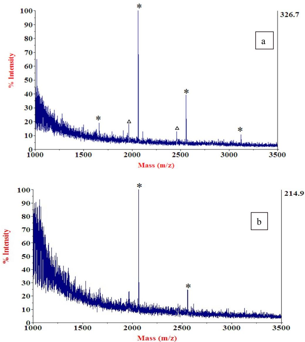
**Fig. S5** MALDI mass spectra of phosphopeptides enrichment by  $\text{Fe}_3\text{O}_4@\text{PDA}@\text{ATP-Ti}^{4+}$  microspheres, with the tryptic digests of  $\beta$ -casein amount as (a) 20 fmol and (b) 2 fmol, where phosphopeptides were marked with \*, and  $\Delta$  indicates the losses of phosphoric acid.
