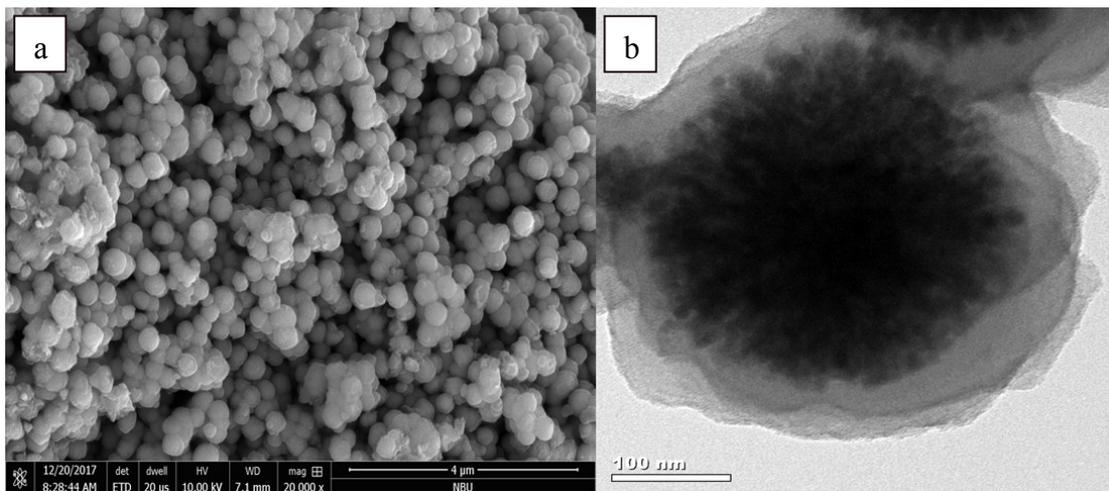
**Fig. S1** Images of (a) SEM and (b) TEM of  $\text{Fe}_3\text{O}_4@\text{PDA}$  microspheres.
