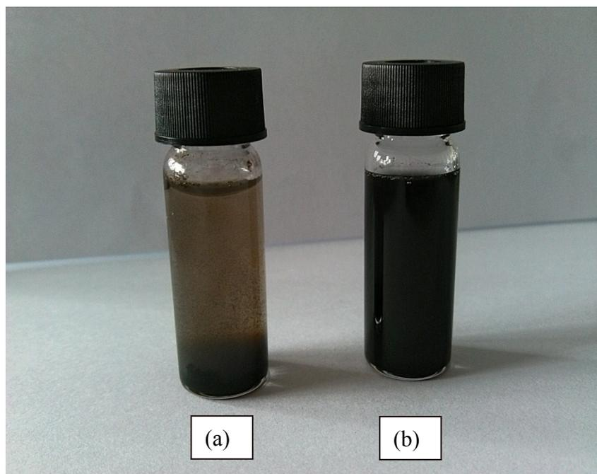
**Fig. S3** Photographs of sample solutions after standing for 30 min (a)  $\text{Fe}_3\text{O}_4$  and (b)  $\text{Fe}_3\text{O}_4@\text{PDA}@\text{ATP-Ti}^{4+}$  microspheres.
