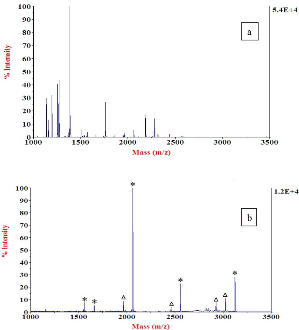
**Fig. S4** MALDI mass spectrum of peptides derived from  $\beta$ -casein (a) before enrichment and (b) after enrichment by  $Fe_3O_4@PDA@ATP-Ti^{4+}$  microspheres, where phosphopeptides were marked with \*, and  $\Delta$  indicates the losses of phosphoric acid.
