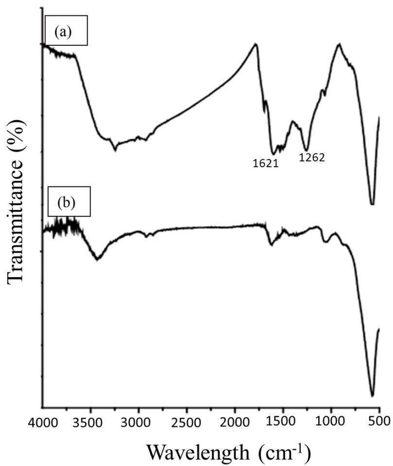
**Fig. S2** FTIR spectrum of (a)  $\text{Fe}_3\text{O}_4@\text{PDA}@\text{ATP-Ti}^{4+}$  and (b)  $\text{Fe}_3\text{O}_4$  microspheres.
