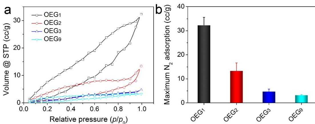
**Fig. S5** a, The  $N_2$  adsorption/desorption curves. b, The maximum  $N_2$  adsorption in OEG xerogels at a maximum relative pressure ( $P/P_0 = 1$ ).
