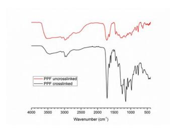
The characteristic peak at 1730 cm<sup>-1</sup> and 1646 cm<sup>-1</sup> corresponded to the ester carbonyl group and unsaturated double bonds in fumarate unit, respectively. Peaks at 1455 cm<sup>-1</sup> and 1375 cm<sup>-1</sup> correspond to methyl stretching, and the peak at 1296 cm<sup>-1</sup> corresponds to the secondary alcohol. These are in a good agreement with literature.<sup>[61]</sup>
