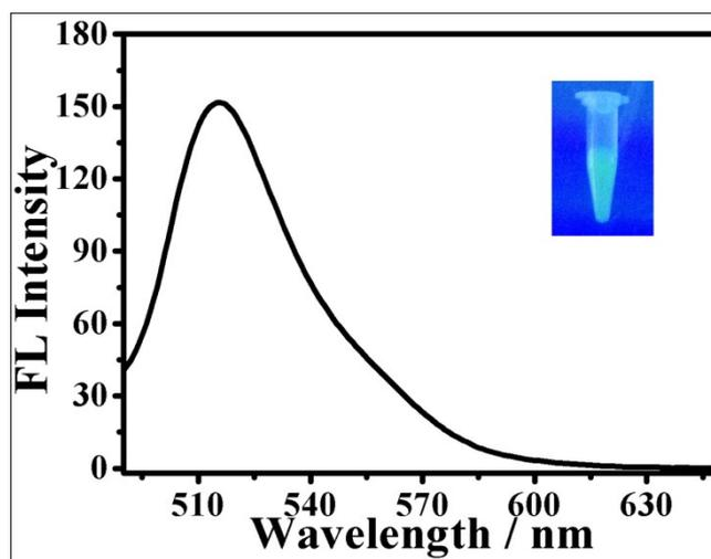
**Figure S14.** The FL emission spectra of FITC modified GO-Se nanocomposites. Inset was the corresponding photograph under the UV plate exposure.
