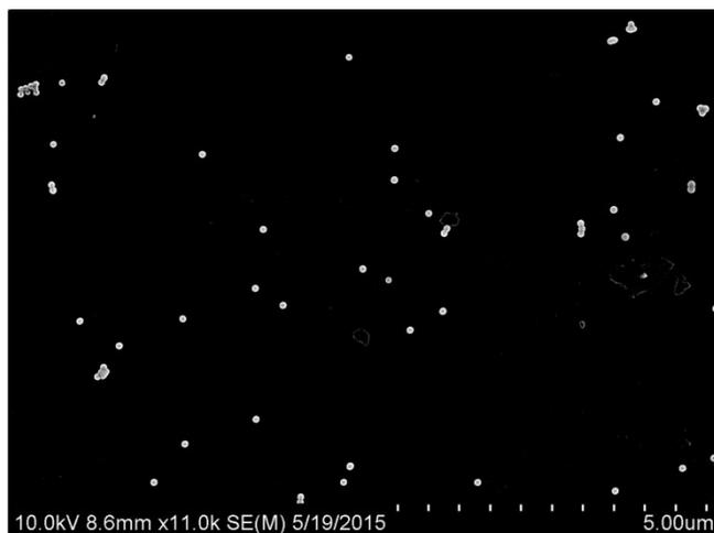
**Figure S9.** The SEM image of Se nanoparticles.
