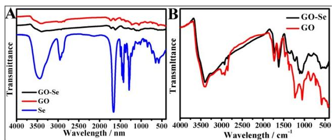
**Figure S6.** A) Fourier Transform Infrared Spectroscopy of GO, Se and GO-Se nanomaterials; B) Fourier Transform Infrared Spectroscopy of GO and GO-Se nanomaterials.
