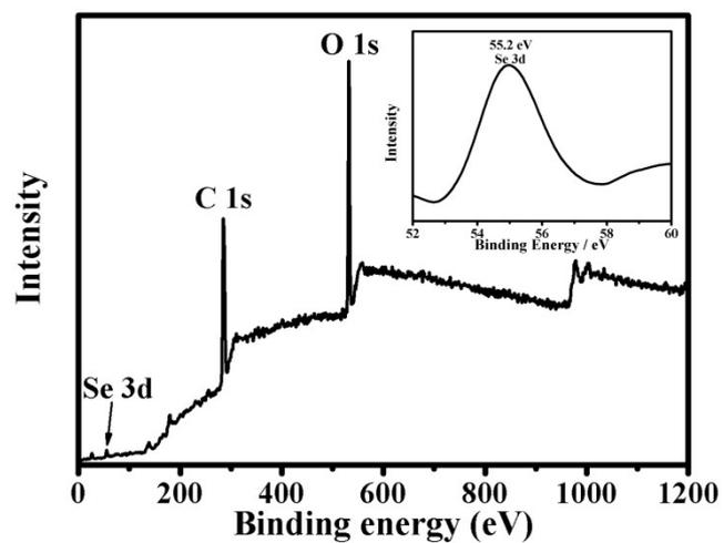
**Figure S5.** XPS spectra of GO-Se nanocomposites. Inset was Se3d spectrum of the nanocomposites.
