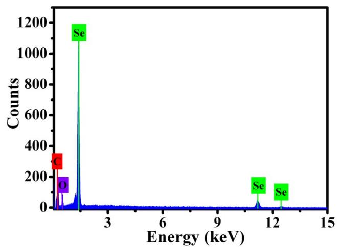
Figure S4. EDX pattern of the GO-Se nanocomposites.
