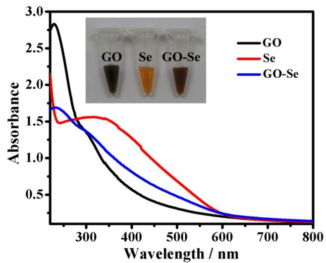
**Figure S8.** UV-Vis spectra of GO, Se and GO-Se nanomaterials. Inset was their corresponding photograph.
