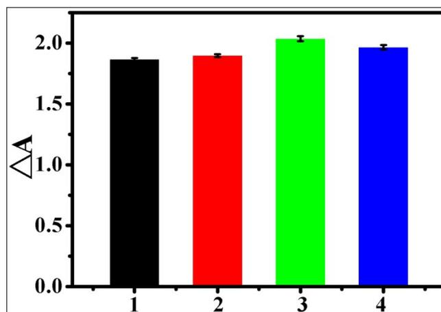
**Figure S13.** The effect of ionic strength and pH on our system: the enzyme-mimic capacities of our nanocomposites were measured under different phosphate buffer. 1) 25 mM pH 7.4; 2) 100 mM pH 7.4; 3) 25 mM pH 5.5; 4) 100 mM pH 5.5.
