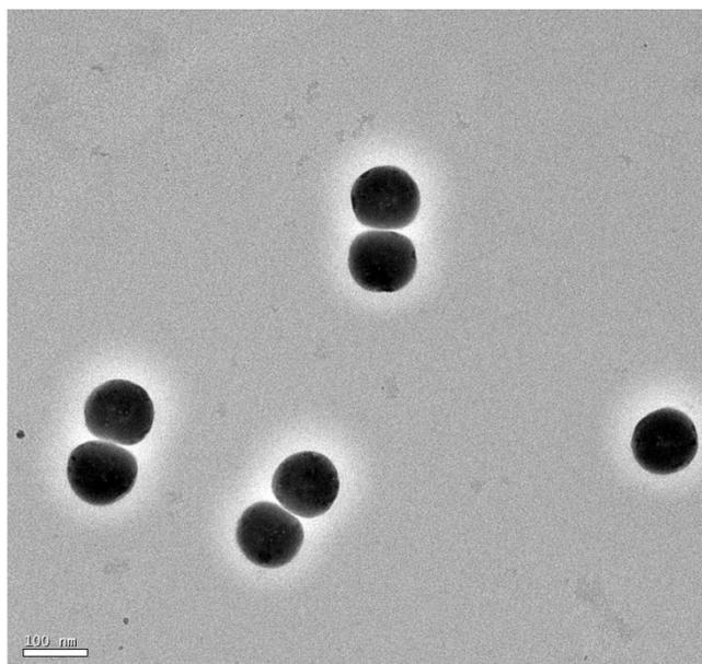
**Figure S10.** The TEM image of Se nanoparticles.
