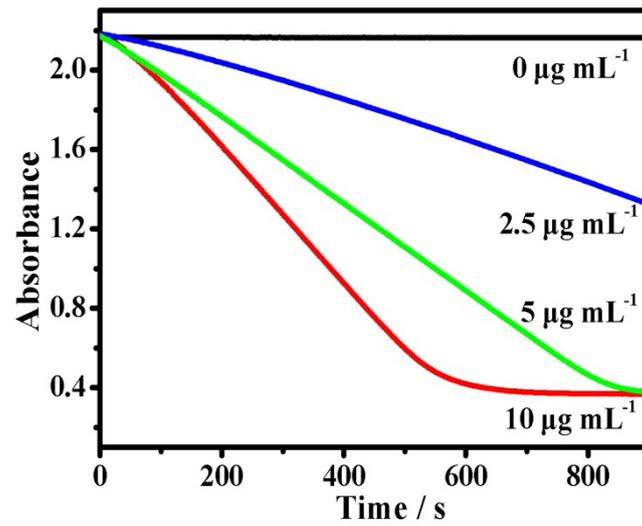
**Figure S11.** Time-dependent absorbance changes of NADPH in the presence of different concentrations of GO-Se nanocomposites.
