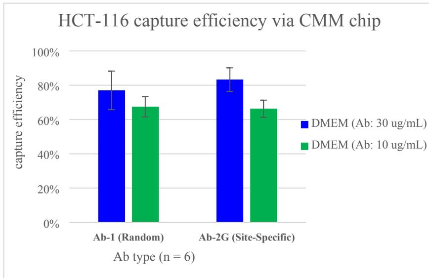
**Figure S7.** The comparison of cell capture efficiency in DMEM with two concentrations (10 or 30  $\mu\text{g/mL}$ ) of two antibodies (**Ab-1** and **Ab-2G**) coated on microfluidic chip surface. The result suggested the concentration 30  $\mu\text{g/mL}$  of antibody was needed to inject onto CMM chip to fill the antibody-biotin-NA binding vacancy on SLB.
