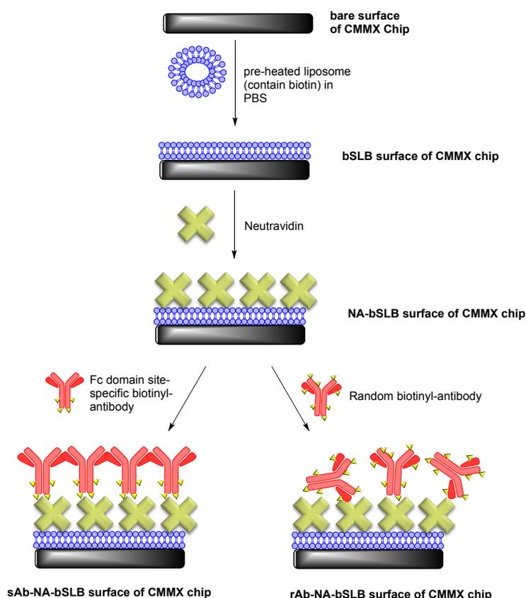
**Figure S3.** Schematic illustration showing reaction steps on formation of anti-EpCAM surface on the SLB of CMM chip.
