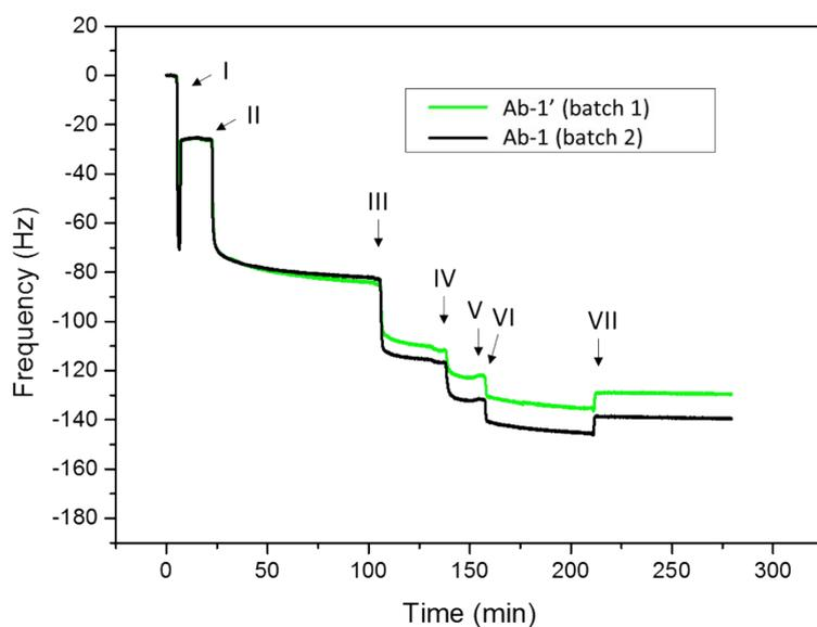
**Figure S6.** The *in situ* QCM kinetic monitoring data for two batches of random biotinylation anti-EpCAM antibodies (**Ab-1** and **Ab-1'**) that has shown different anti-EpCAM loading amount and corresponding EpCAM antigen recognition ability.
