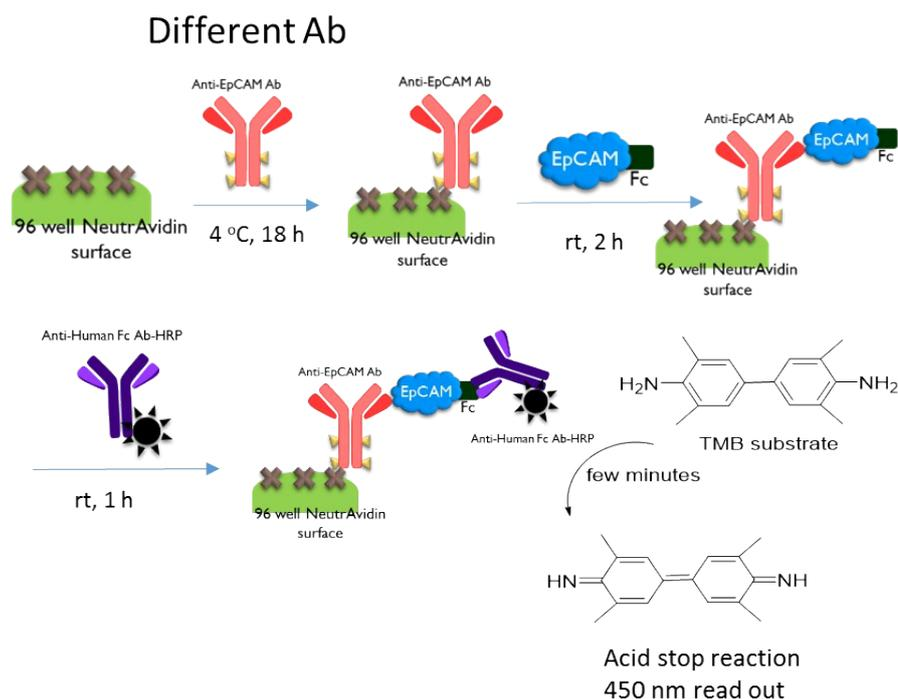
**Figure S4.** Schematic illustration of ELISA assay principal for the ability of diverse biotinyl anti-EpCAM in recognizing its antigen.
