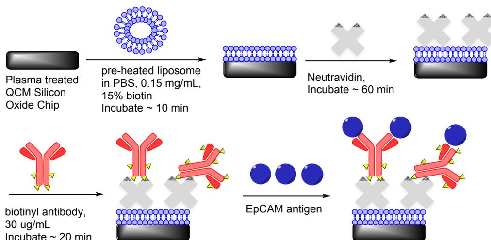
**Figure S5.** Schematic illustration of Quartz Crystal Microgravimetry (QCM) assay including steps on formation and coating of each later.
