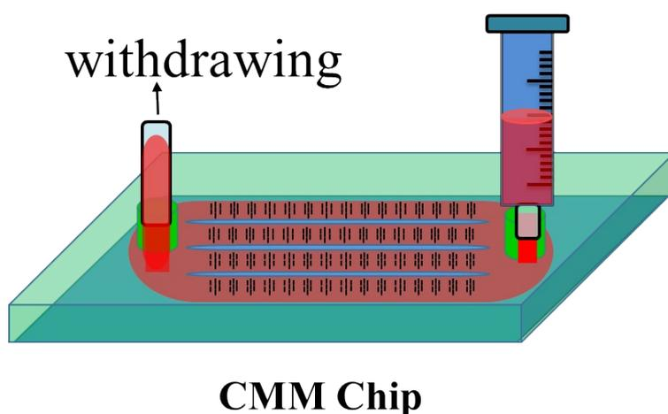
**Figure S2.** An illustration of chaotic mixing microfluidic (CMM) chip. Syringe loaded with 2 mL blood and connected at the inlet of the chip. The blood sample will then be processed through the microfluidic channel on the CMM chip by syringe pump withdrawal. CMM chip has slight modification from CMx chip.<sup>R3-4</sup>
