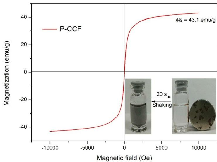
**Fig. S4.** Hysteresis loop of P-CCF and the dispersion and separation process of P-CCF (inset).
