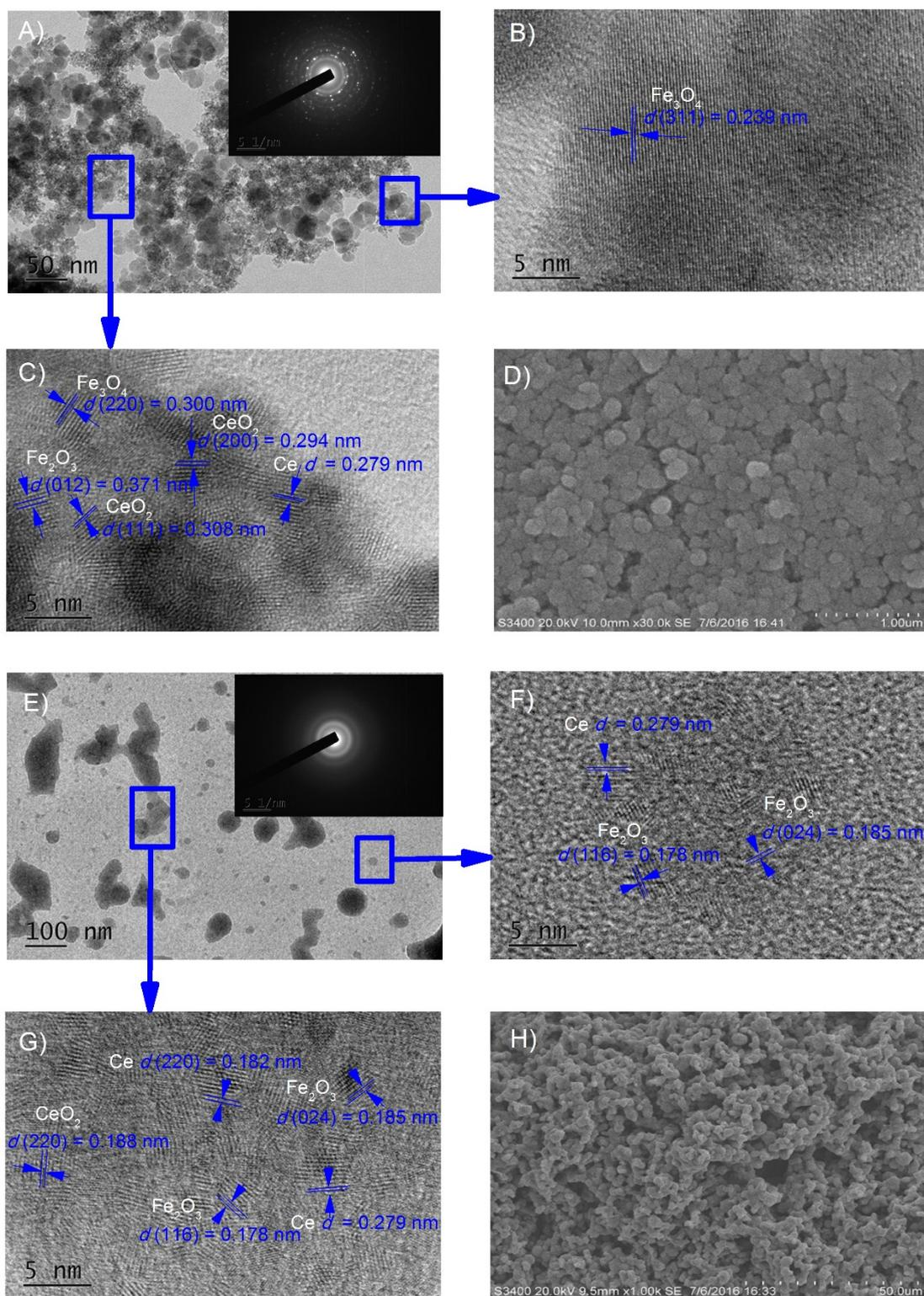
**Fig. S2.** TEM images (A and E), SAED patterns (A and E, inset), HRTEM images for different areas (B, C, F and G) and SEM images (D and H) of P-CCF (A-D) and CSF (E-H), respectively.
