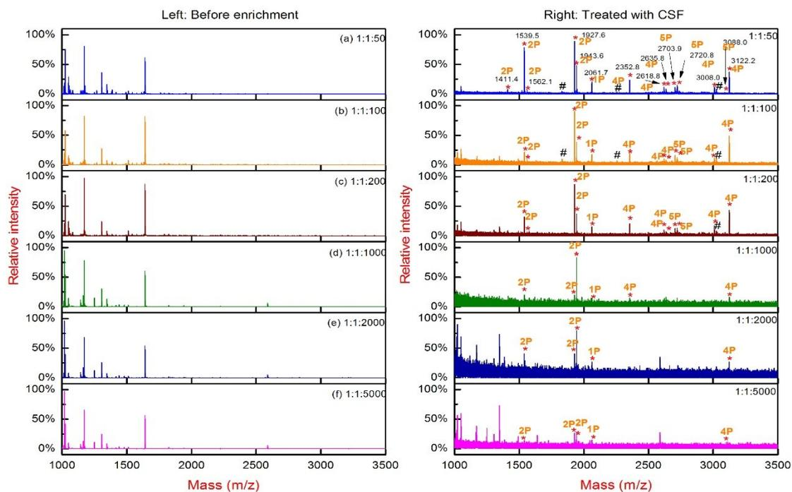
**Fig. S6.** MALDI-TOF MS spectra of tryptic digests of bovine  $\alpha$ - and  $\beta$ -casein and BSA at mass ratios of 1:1:50, 1:1:100, 1:1:200, 1:1:1000, 1:1:2000, and 1:5000 treated without (Left: a-f) and with (Right) CSF affinity probe. Phosphorylations were labelled as P. Arabic numeral before P represents mono-/multi-phosphopeptides. “\*” indicates phosphopeptides; “#” indicates the dephosphorylated fragments of phosphopeptide.
