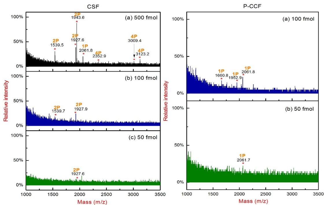
**Fig. S5.** MALDI-TOF MS spectra of mixture of bovine  $\alpha$ - and  $\beta$ -casein digests treated with CSF (Left) and P-CCF (Right), respectively. Left: (a). 500 fmol; (b). 100 fmol; (c). 50 fmol; Right: (a) 100 fmol; (b) 50 fmol. Phosphorylations were labelled as P. Arabic numeral before P represents mono-/multi-phosphopeptides. “\*” indicates phosphopeptides; “#” indicates the dephosphorylated fragments of phosphopeptide.
