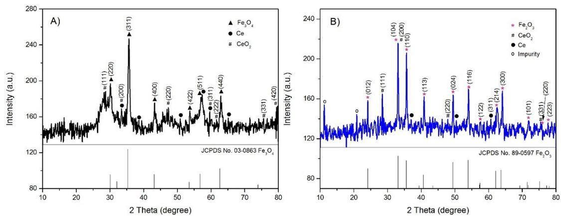
**Fig. S3.** XRD patterns of P-CCF (A) and CSF (B).
