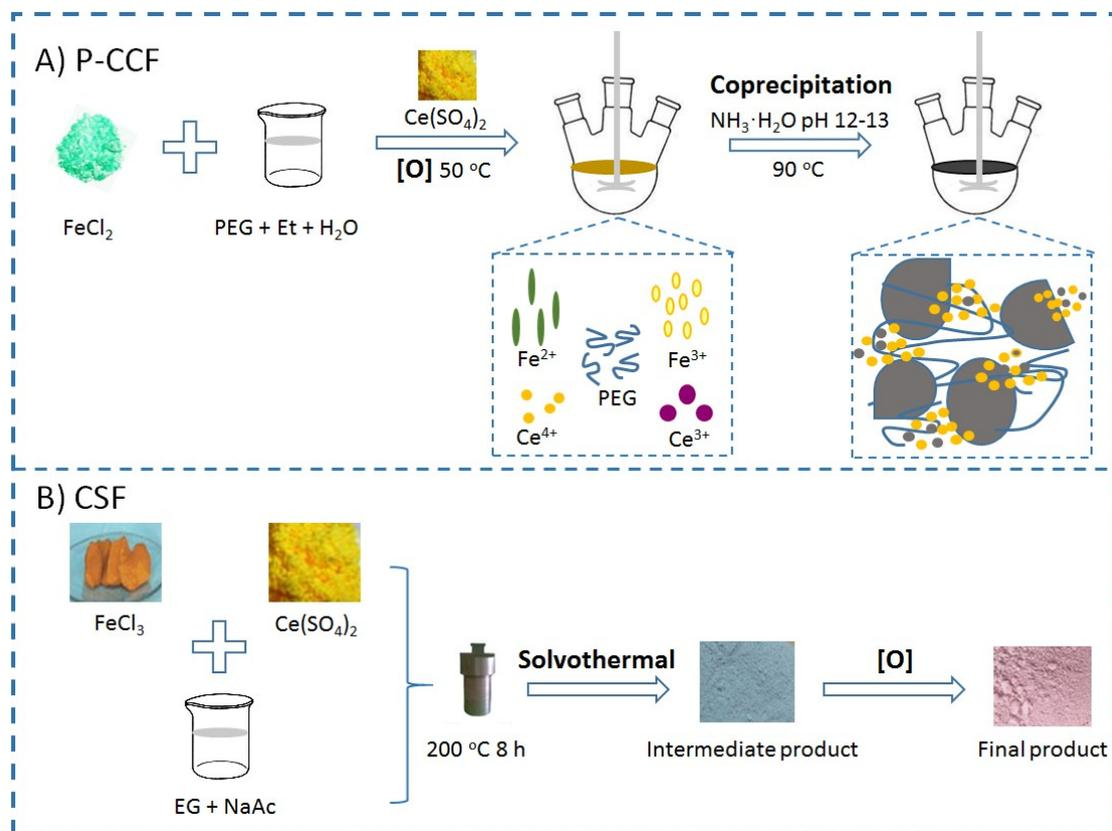
**Scheme S1.** Synthesis of P-CCF (A) and CSF (B).
