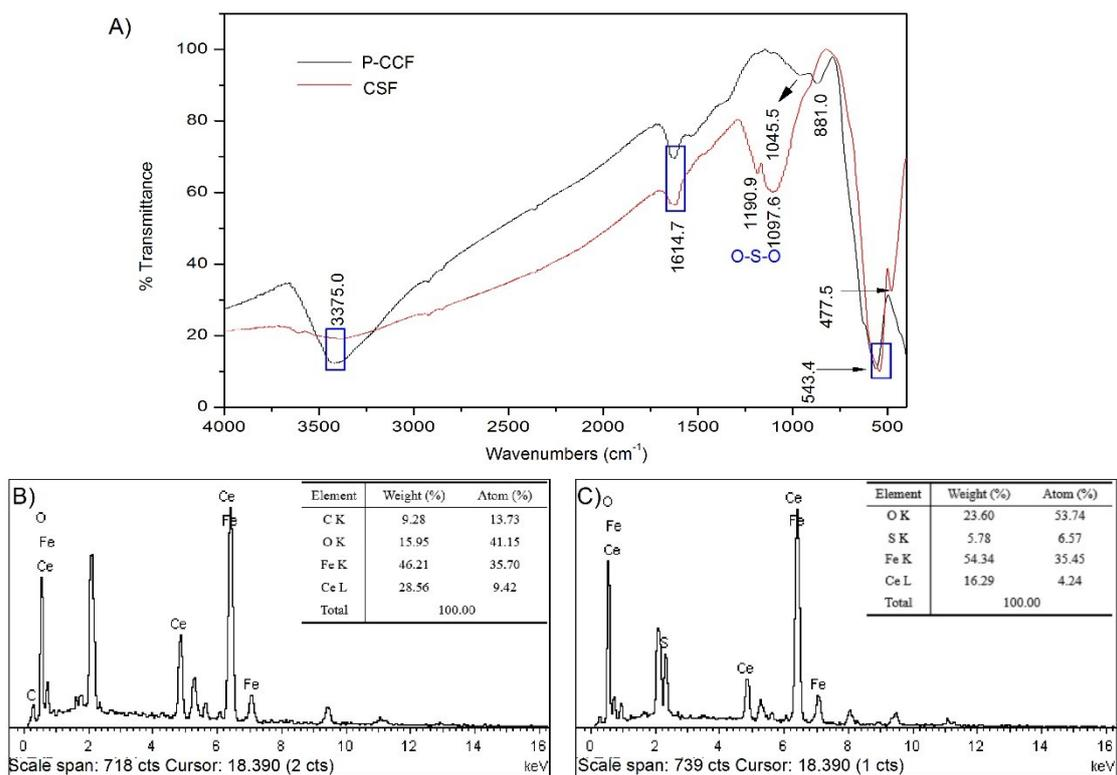
**Fig. S1.** FT-IR spectra (A) of P-CCF (black line) and CSF (red line), and EDX spectra of P-CCF (B) and CSF (C).
