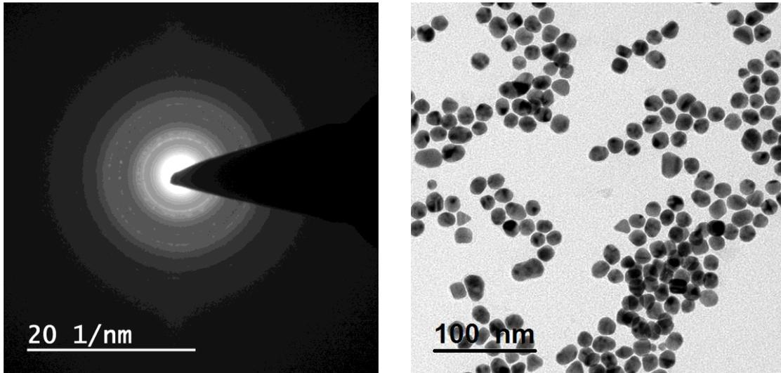
**Figure S9.** SAD (left) and TEM (right) images of Au-4
