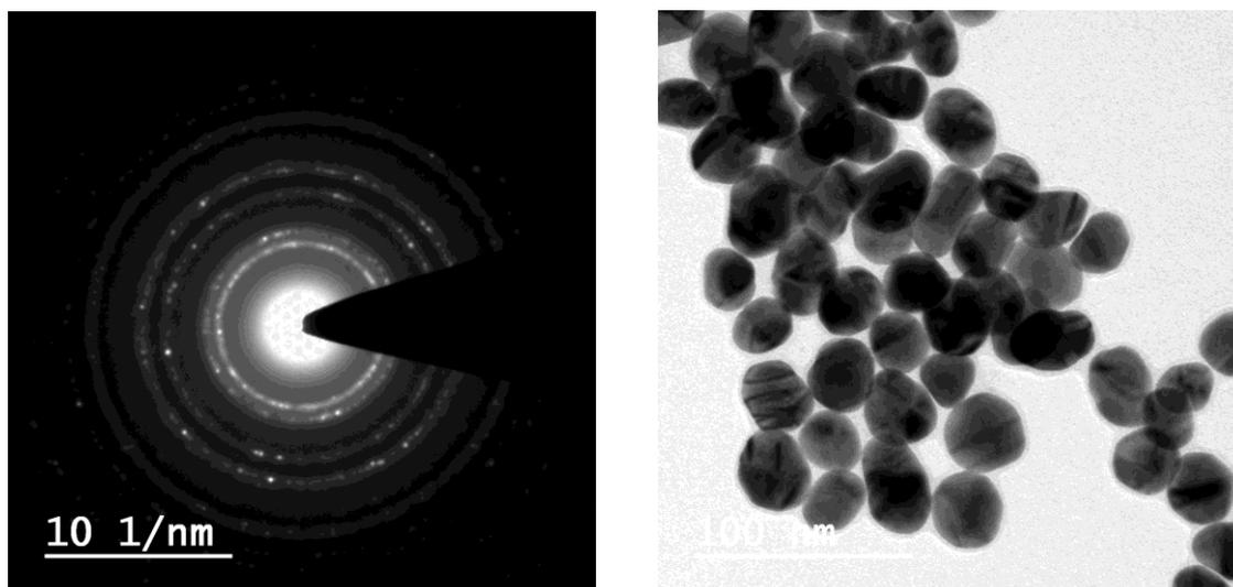
**Figure S1.** SAD (left) and TEM (right) image of Au-1.
