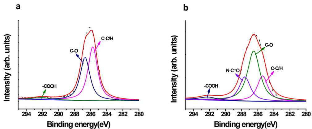
**Fig. S4** The measured C(1s) core level XPS spectra of (a) Au NCs and (b) nanoprobe.
