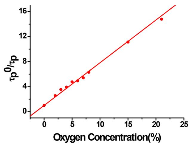
**Fig. S6** The corresponding Stem–Volmer plot of  $\tau_p^0 / \tau_p$  against the partial pressure of oxygen. The ratios between the phosphorescence lifetime of complex **1** and the lifetime of Au NCs in the absence and presence of O<sub>2</sub> are defined as  $\tau_p^0$  and  $\tau_p$ . The  $K_{sv}$  was calculated to be 0.68%<sup>-1</sup>, which was in accordance to the results obtained from ratio.
