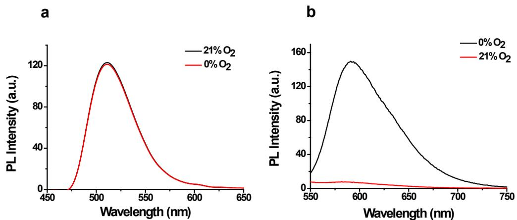
**Fig. S1** (a) The photoluminescence spectra of Au NCs in PBS buffer (pH = 7.4) under 21% and 0% O<sub>2</sub> degree; (b) The photoluminescence spectra of iridium(II) complex **1** in DMSO under 21% and 0% O<sub>2</sub> degree.
