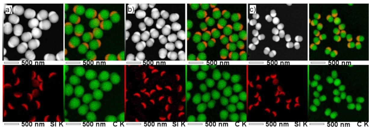
**Figure S6.** TEM-EDS images of polystyrene particles ( $d=386$  nm (a), 338 nm (b), 218 nm (c)) with polyphenylsiloxane caps synthesized with 13  $\mu$ L Ph-TMS.
