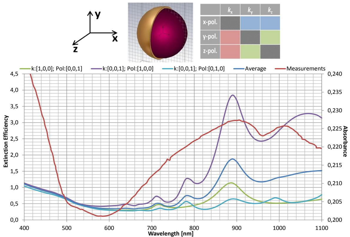
**Figure S3.** UV/VIS measurements and theoretical calculations using finite element method of Au semishells after deprotection.
