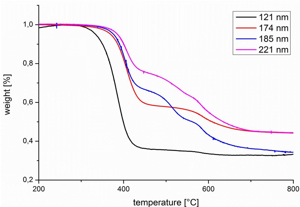
**Figure S5.** TGA measurements of polystyrene-polyphenylsiloxane composite particles with core diameter of 281 nm and different cap sizes.
