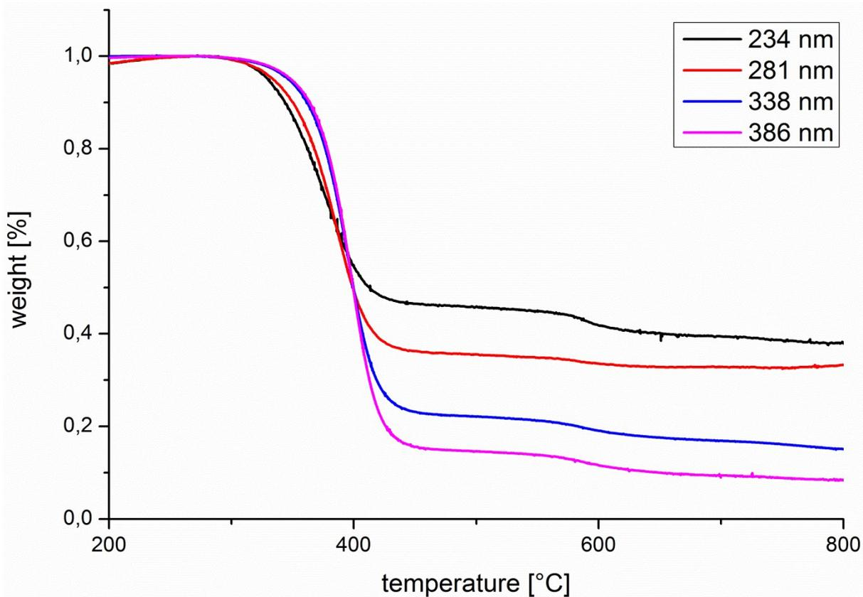
**Figure S7.** TGA measurements of polystyrene-polyphenylsiloxane composite particles with different core diameters nm and cap sizes around 130 nm (radius).
