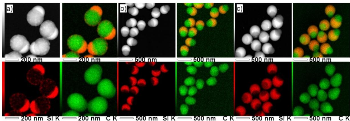
**Figure S4.** TEM-EDS images of polystyrene particles ( $d=281$  nm) with polyphenylsiloxane caps of various sizes synthesized with a) 13  $\mu$ L, b) 50  $\mu$ L and c) 120  $\mu$ L Ph-TMS.
