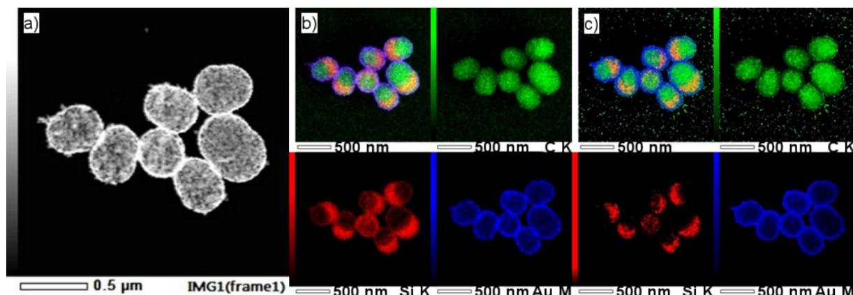
**Figure S1.** a) TEM image, b) raw count and c) quantified EDS mappings of polystyrene-polyphenylsiloxane composite particles plated with a thin Au shell (nanoshells). The thin Si shell that seems to be present around the entire polystyrene part in the raw count EDS mapping is an artefact due to partial peak overlap between the Si-K $\alpha$  line and the Au-M $\alpha$  line.
