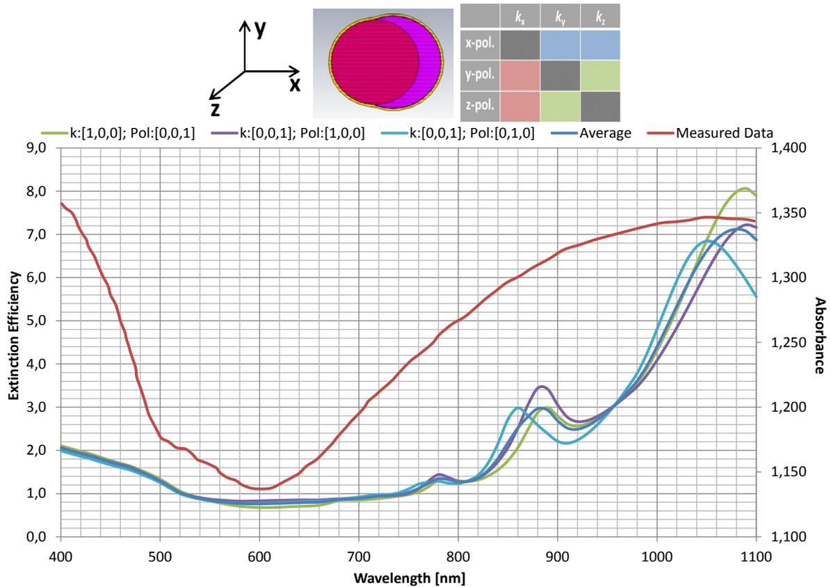
**Figure S2.** UV/VIS measurements and theoretical calculations using finite element method of polystyrene-polyphenylsiloxane composite particles plated with a thin Au shell (nanoshells).
