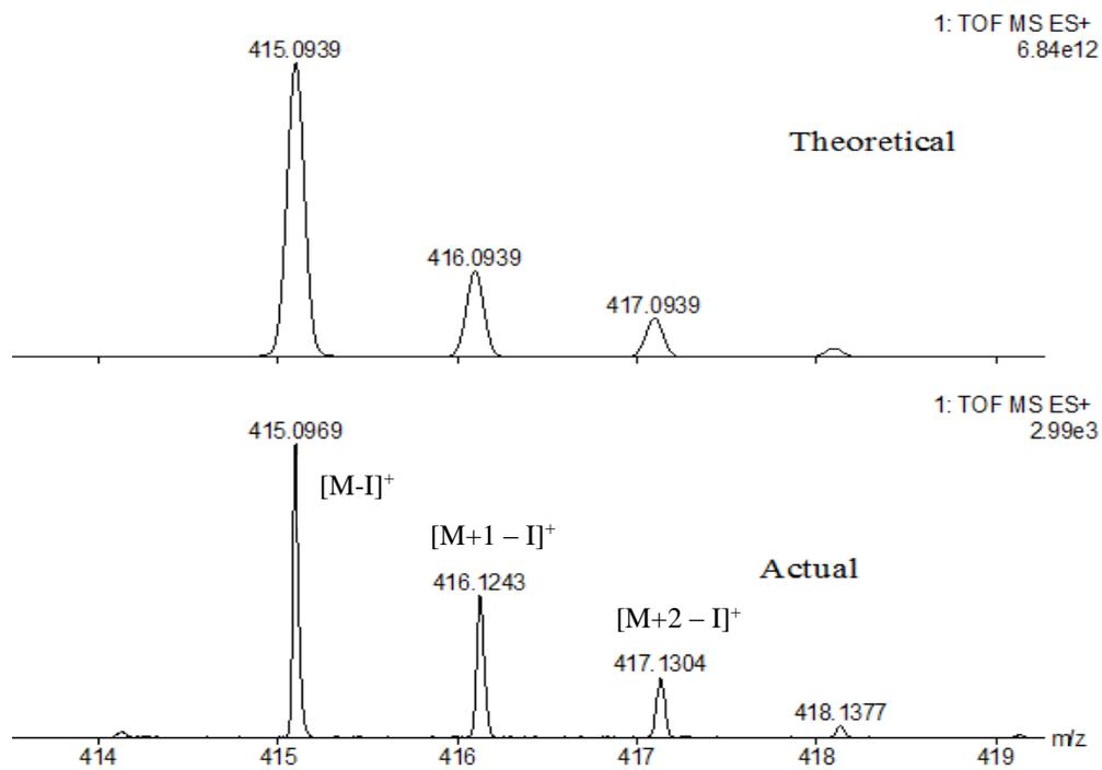
Figure S10: TOF MS ES<sup>+</sup> Mass Spectra of **8**.
