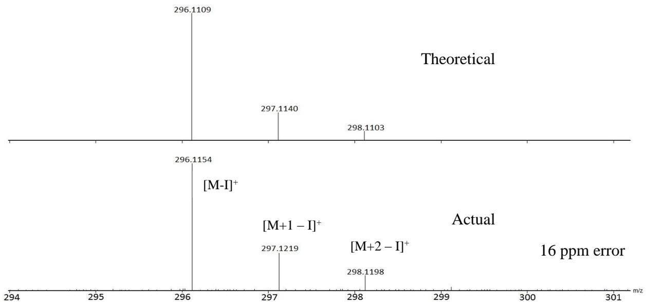
Figure S9: TOF MS ES<sup>+</sup> Mass Spectra of **3**.
