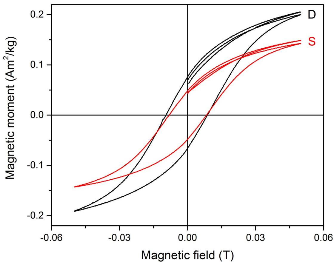
**Figure S1.** Magnetization versus field curves for magnetic zeolite samples. D-Dynamic, S-Static.
