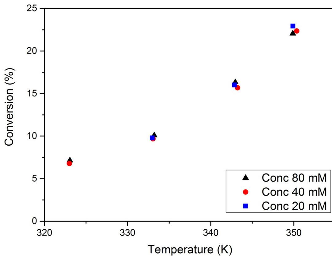
**Figure S5.** Light-off curves for citronellal isomerisation. Catalyst weight: 82.2 mg. Liquid flow rate: 0.1 ml/min. Gas flow rate: 3.0 ml/min (STP).
