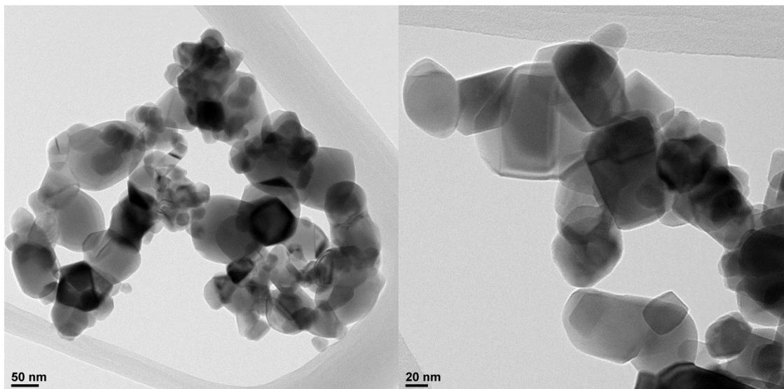
**Figure S2.** TEM micrographs  $\text{TiO}_2$ -coated ferrite nanoparticles synthesized in this study.
