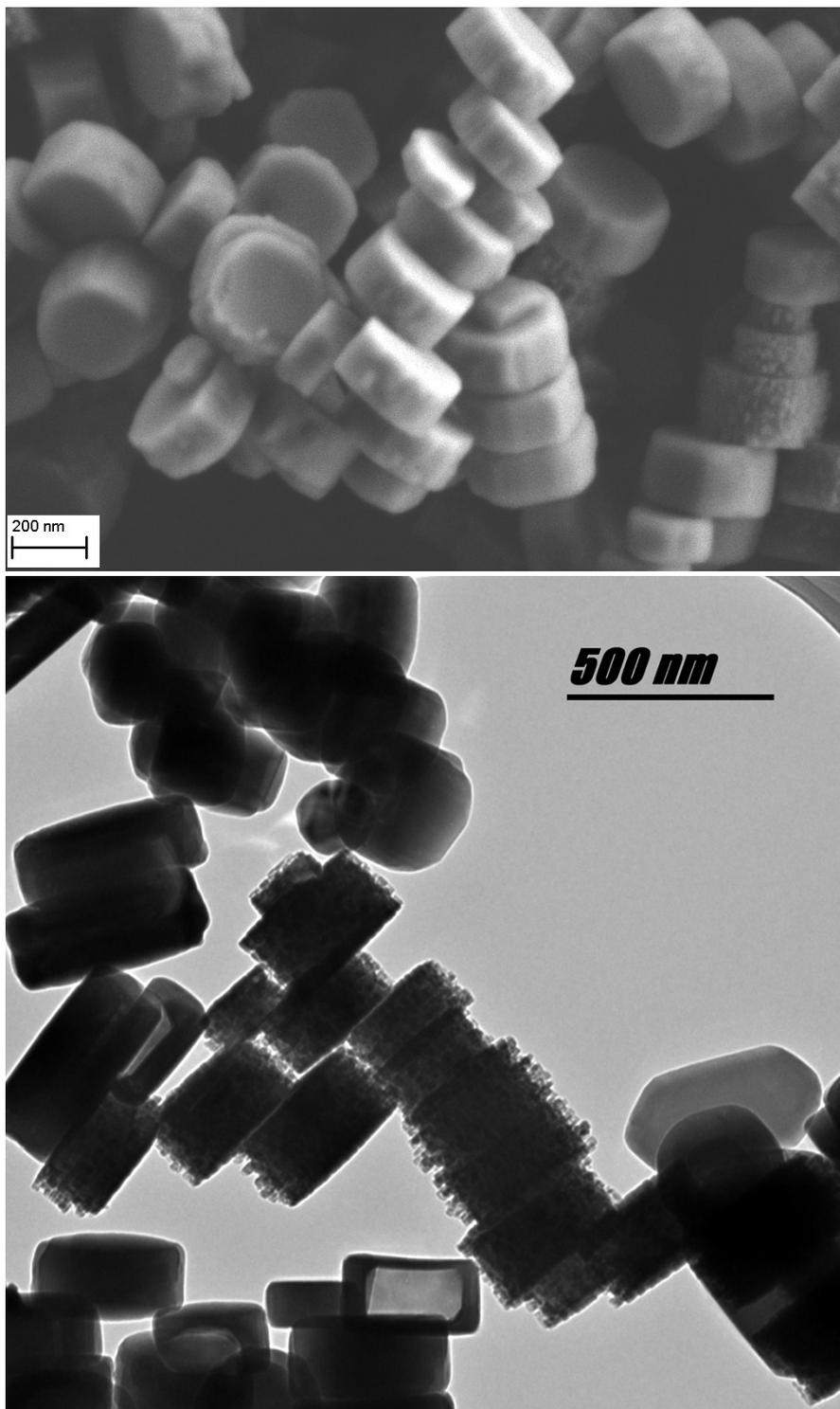
**Figure S3.** FE-SEM (top) and TEM (bottom) pictures of the ferrite@zeolite nanoparticles synthesized under static conditions at 438 K for 5 days.
