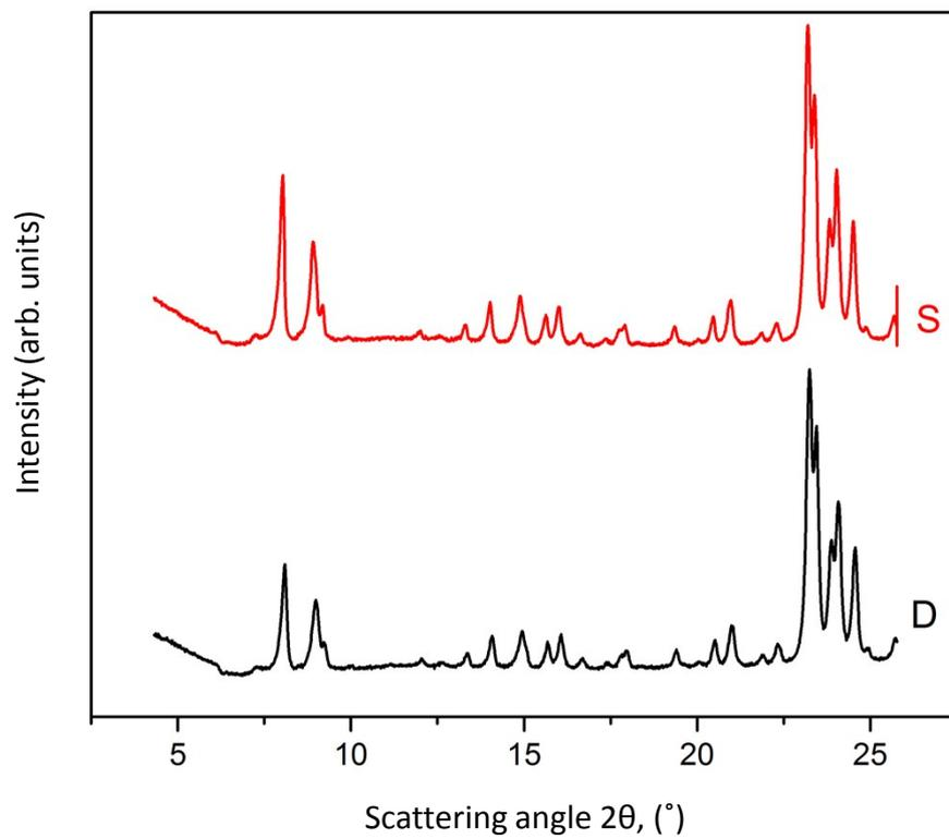
**Figure S4.** Powder x-ray diffraction patterns of magnetic zeolite. D-Dynamic, S-Static.
