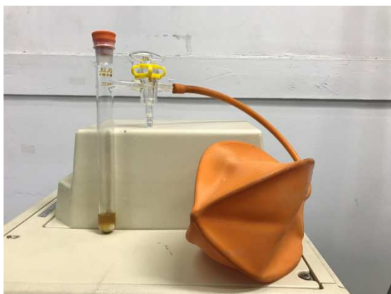
Fig. S2 The reactor used in this study. The balloon was partially filled with Ar gas.
