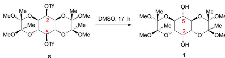
Precipitation by addition of water (0.5 mL) after 17 h gave the diol **1** (25 mg, 85 %) as a white solid.
