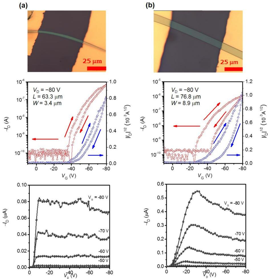
**Fig. S5** Optical micrographs (top panels), transfer characteristics (middle panels), and output characteristics of representative OFETs based on microribbons of (a) **2** and (b) **3**.
