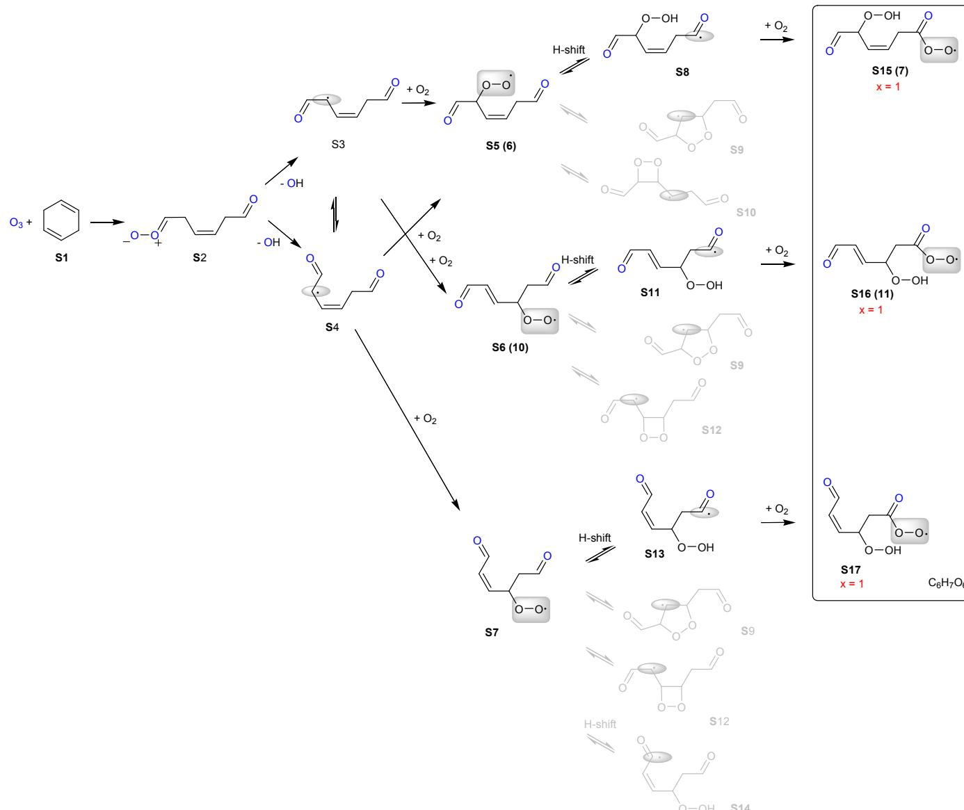
*Scheme S1* First reaction steps of the ozonolysis of 1,4-CHD. Oxygen atoms arising from the attacking ozone are highlighted in blue, alkyl radical functional groups with a shaded oval and  $\text{RO}_2$  radical functional groups with a shaded rectangle. Detected species are surrounded by a solid rectangle. Species in grey (**S9**, **S10**, **S12** and **S14**) are not significantly formed according to the calculations. The numbering in brackets belongs to the numbering in the main text.
