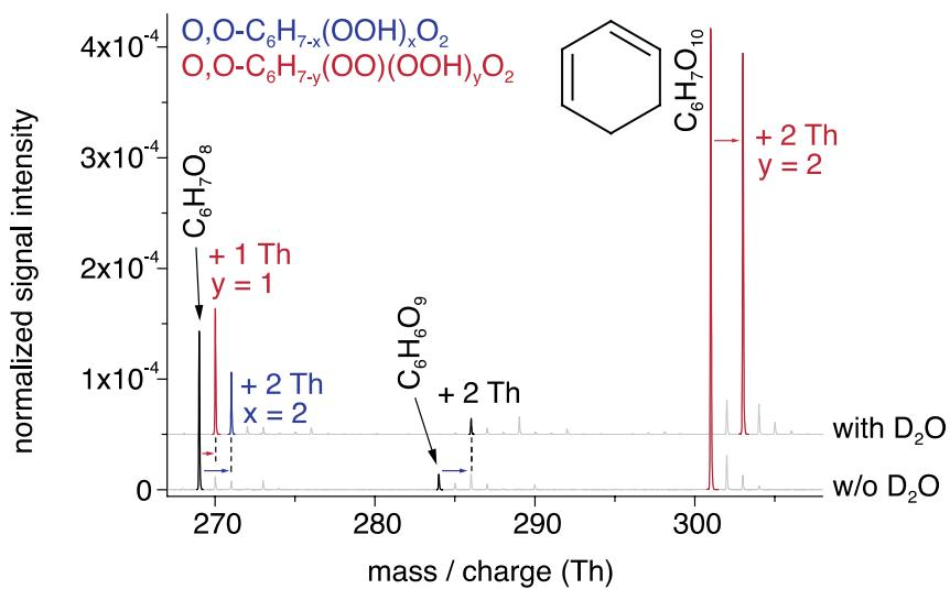
Fig. S2 Comparison of mass spectra from the ozonolysis of 1,3-cyclohexadiene recorded either in the absence (lower spectrum) or presence (upper spectrum) of heavy water used for H/D exchange of acidic H atoms.
