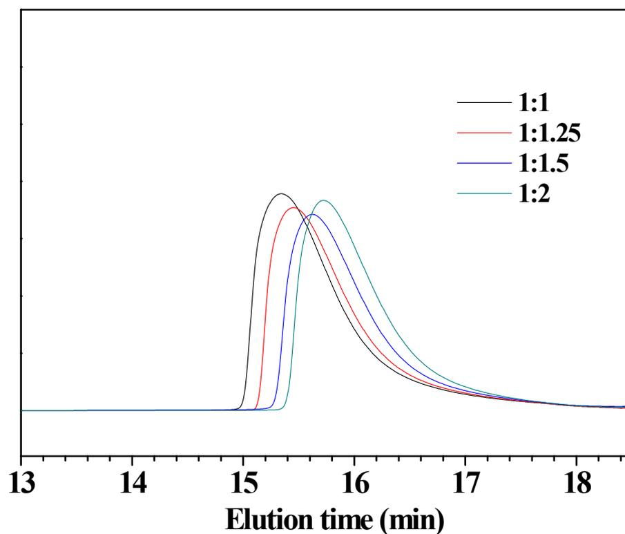
**Figure S2.** GPC profiles of PBLG with varying the molar ratio of  $\text{Fmes}_2\text{BF}$  and aniline as initiator.  $[\text{Fmes}_2\text{BF}]/[\text{aniline}] = 1/1 \sim 1/2$ ,  $[\text{Glu-NCA}] = 0.5\text{ M}$ , at  $25\text{ }^\circ\text{C}$  in DCM.
