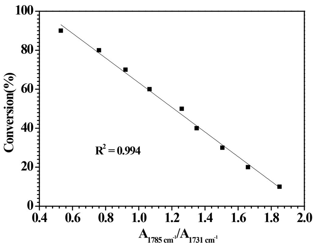
**Figure S1.** Calibrated curve of Glu-NCA conversion vs the peak intensity ratio at  $1785\text{ cm}^{-1}$  and  $1731\text{ cm}^{-1}$ .
