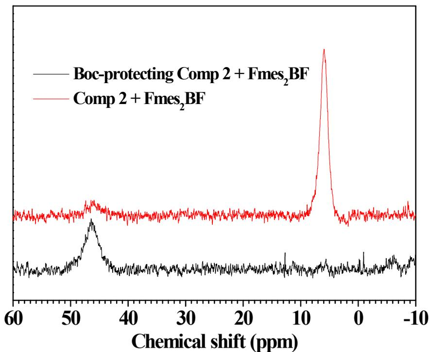
**Figure S9.** <sup>11</sup>B NMR spectra of Fmes<sub>2</sub>BF and  $\alpha$ -amino- $\beta$ -benzyl-L-aspartamyl aniline before and after Boc removal with molar ratio of 1 to 1.
