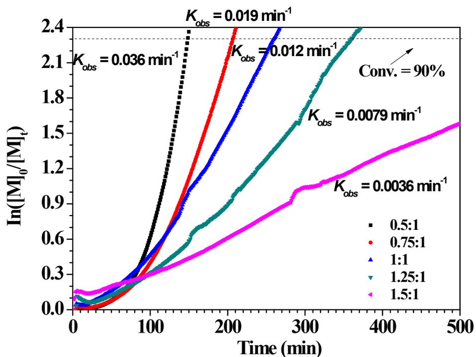
**Figure S5.** Kinetics of the ROP of Glu-NCA initiated by the aniline and Fmes<sub>2</sub>BF system ([Glu-NCA] = 0.50 M, [Glu-NCA]/[aniline] = 50, [Fmes<sub>2</sub>BF]/[aniline] = 0.5, 0.75, 1.0, 1.25 and 1.5, 25 °C in DCM, the automatic sampling interval of *in situ* IR is 60 seconds).
