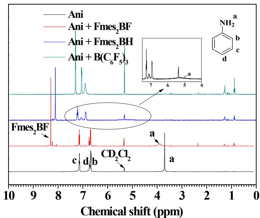
**Figure S3.**  $^1\text{H}$  NMR spectra of chemical structures of aniline interacting with  $\text{Fmes}_2\text{BF}$ ,  $\text{Fmes}_2\text{BH}$  and  $\text{B}(\text{C}_6\text{F}_5)_3$ .
