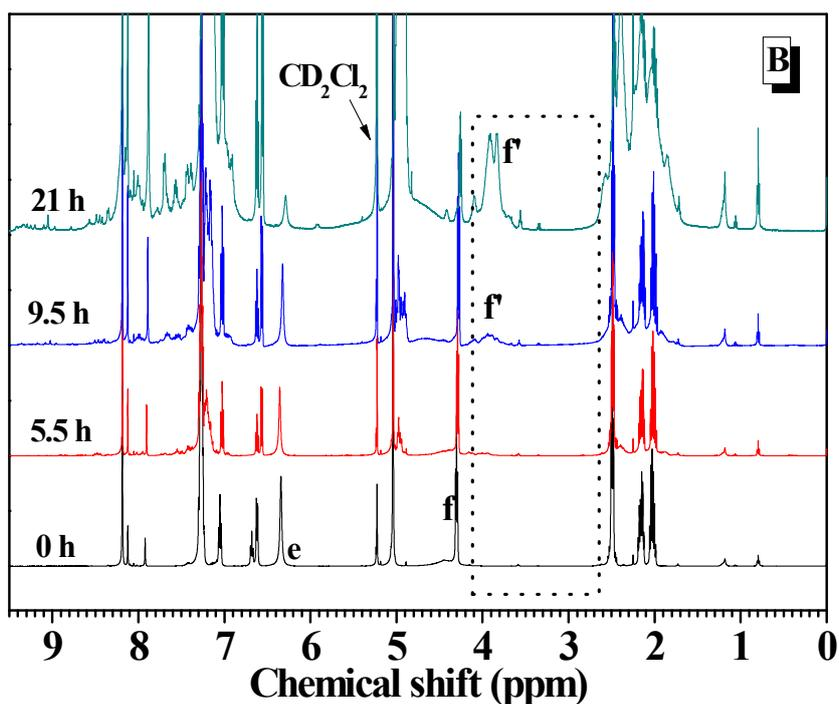
**Figure S10.**  $^1\text{H}$  NMR spectra of polymerization process of Glu-NCA in the presence of aniline,  $[\text{Glu-NCA}]/[\text{aniline}] = 5/1$  (A); in the presence of FLPs consisting of  $\text{Fmes}_2\text{BF}$  and aniline (B),  $[\text{Glu-NCA}]/[\text{aniline}]/[\text{Fmes}_2\text{BF}] = 5:1:1$ ,  $25^\circ\text{C}$  in  $\text{CD}_2\text{Cl}_2$ .
