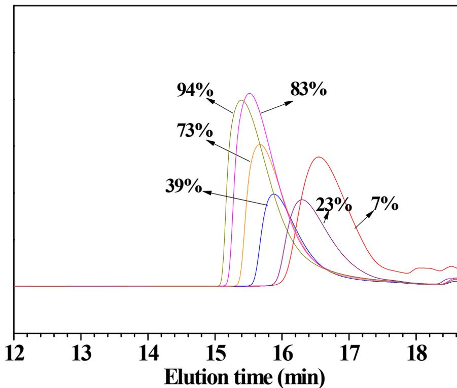
**Figure S6.** GPC profiles of PBLG depending on the different monomer conversion. [Glu-NCA]/[Fmes<sub>2</sub>BF]/[aniline] = 50/1/1, [Glu-NCA] = 0.5 M, at 25 °C in DCM.
