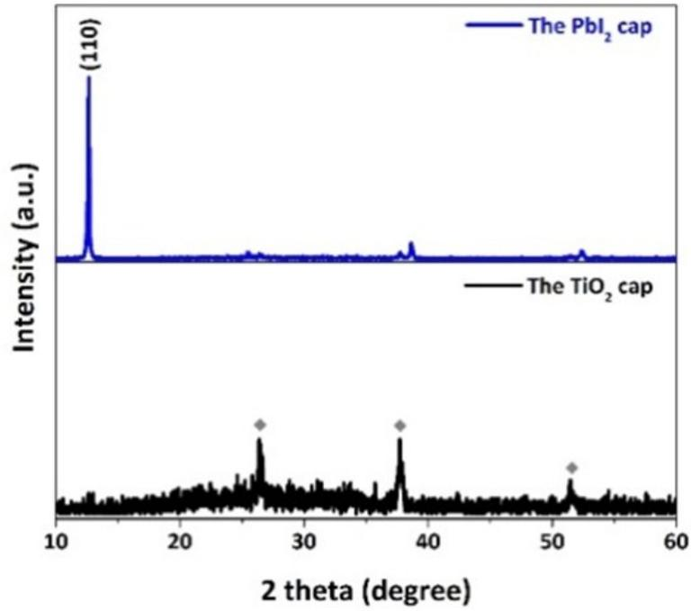
Fig. S5 XRD patterns of the Pbl<sub>2</sub> and TiO<sub>2</sub> cap respectively. The diamond symbols are corresponding to the signals from the TiO<sub>2</sub>/FTO substrate.
