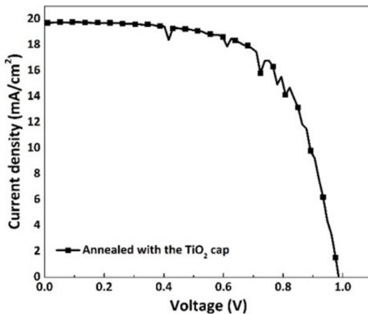
Fig. S13 Optimized J-V curve of the fabricated perovskite solar cell with the CH<sub>3</sub>NH<sub>3</sub>PbI<sub>3</sub> perovskite film annealed with the TiO<sub>2</sub> cap.
