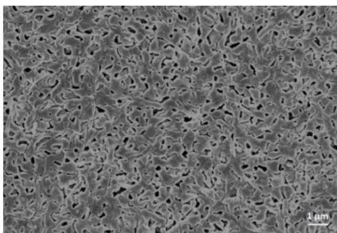
**Fig. S9** Top-view SEM image of the  $\text{PbI}_2$  cap.
