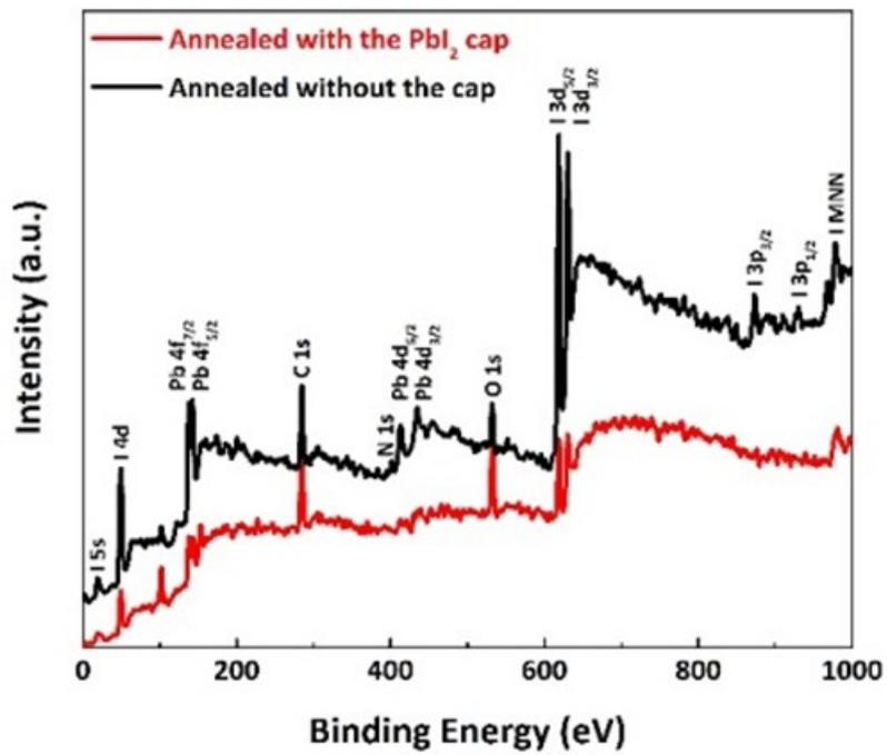
Fig. S6 XPS spectra of the CH<sub>3</sub>NH<sub>3</sub>PbI<sub>3</sub> perovskite films annealed with and without the Pbl<sub>2</sub> cap.
