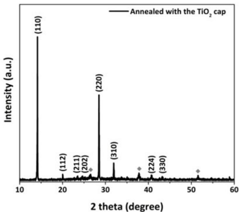
**Fig. S4** XRD pattern of the CH<sub>3</sub>NH<sub>3</sub>PbI<sub>3</sub> perovskite film annealed with the TiO<sub>2</sub> cap. The diamond symbols are corresponding to the signals from the TiO<sub>2</sub>/FTO substrate.
