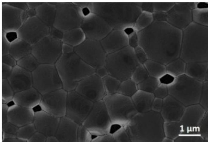
**Fig. S7** Top-view SEM image of the  $\text{CH}_3\text{NH}_3\text{PbI}_3$  perovskite film annealed with the  $\text{TiO}_2$  cap.
