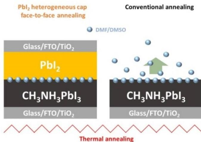
**Fig. S16** Diagram of the residual DMF or DMSO solvent molecules at the interface between the PbI<sub>2</sub> heterogeneous cap and the CH<sub>3</sub>NH<sub>3</sub>PbI<sub>3</sub> perovskite film during the PbI<sub>2</sub> heterogeneous cap face-to-face annealing process. The blue balls are sketches of DMF or DMSO solvent molecules.
