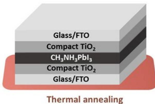
**Fig. S3** Diagram of the TiO<sub>2</sub> heterogeneous cap face-to-face annealing process where the CH<sub>3</sub>NH<sub>3</sub>PbI<sub>3</sub> perovskite film is covered face-to-face with a TiO<sub>2</sub> heterogeneous cap during thermal annealing.
