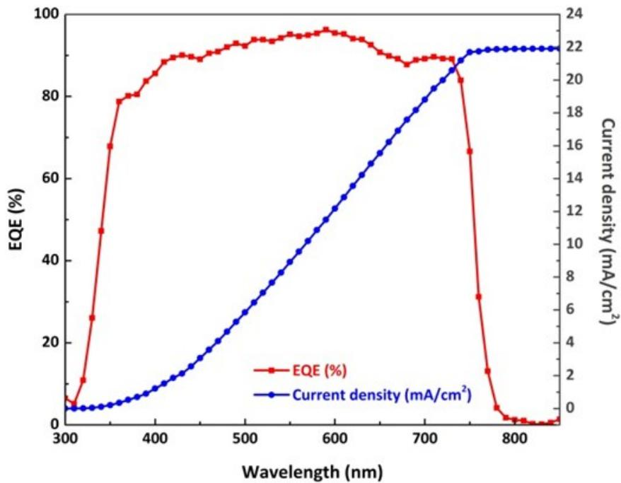
**Fig. S15** EQE curve taken with the monochromatic light without applied white-light bias and correspondingly calculated J<sub>sc</sub> curve of the optimized perovskite solar cell with the CH<sub>3</sub>NH<sub>3</sub>PbI<sub>3</sub> perovskite film annealed with the PbI<sub>2</sub> cap.
