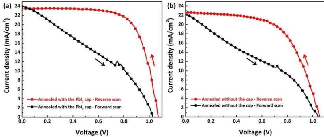
**Fig. S14** J-V curves measured at reverse scan (1.2 V to -0.1 V) and forward scan (-0.1 V - 1.2 V) of the fabricated perovskite solar cell with the CH<sub>3</sub>NH<sub>3</sub>PbI<sub>3</sub> perovskite films annealed (a) with and (b) without the PbI<sub>2</sub> cap.
