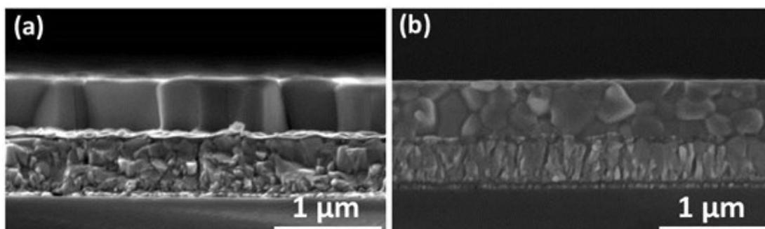
**Fig. S8** Cross-sectional SEM images of the  $\text{CH}_3\text{NH}_3\text{PbI}_3$  perovskite films annealed with (a) and (b) without the  $\text{PbI}_2$  cap.
