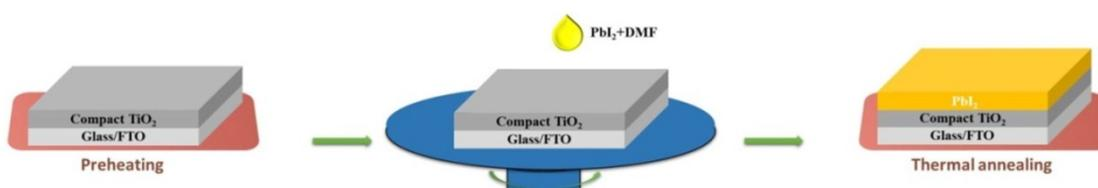
**Fig. S2** Diagram of the preparation of the PbI<sub>2</sub> heterogeneous cap.
