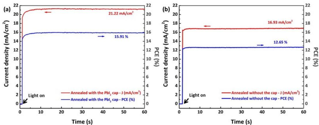
Fig. S12 Stabilized current density and PCE output (measured at 0.75 V) of the fabricated perovskite solar cells annealed with the CH<sub>3</sub>NH<sub>3</sub>PbI<sub>3</sub> perovskite films (a) with and (b) without the PbI<sub>2</sub> cap.
