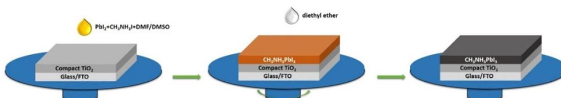
**Fig. S1** Diagram of the preparation of the CH<sub>3</sub>NH<sub>3</sub>PbI<sub>3</sub> perovskite film.
