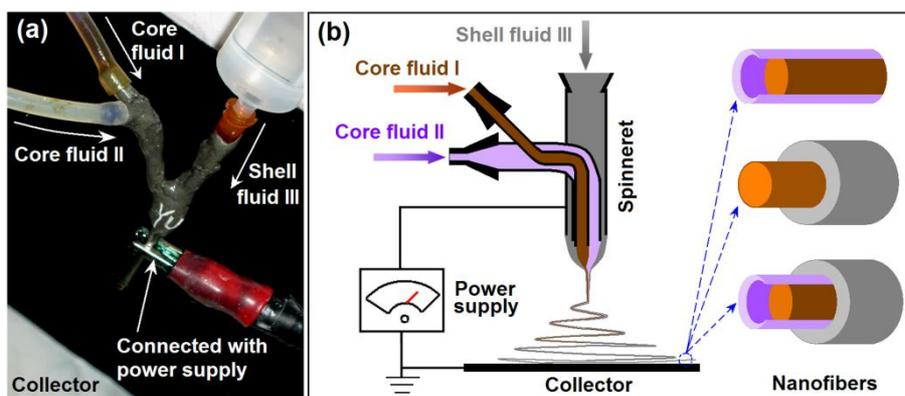
**Figure S6.** (a) A digital photo of the connection of the structured spinneret and its connections with the power supply and syringe pumps; (b) The exploitation of the structured spinneret for the fabrication of different kinds of nanostructures, including core-shell, Janus and core-shell with Janus core structures.
