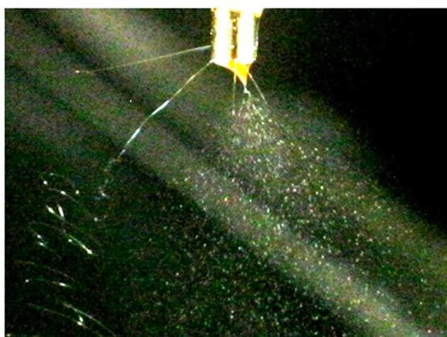
**Figure S1.** Preparation of Janus nanofibers with 8% w/v PVP and 30% w/v shellac solutions, using the parallel spinneret I. The two fluids can be seen to separate at the point of exiting the spinneret, with each having its own Taylor cone.
