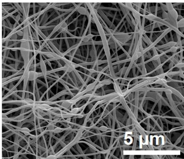
**Figure S4.** Nanofibers prepared with 8% w/v PVP and 30% w/v shellac solutions using the acentric spinneret II. The products are observed to be a combination of fibers and particle-fiber structures consisting of shellac and PVP K60, with some separation of the two sides.
