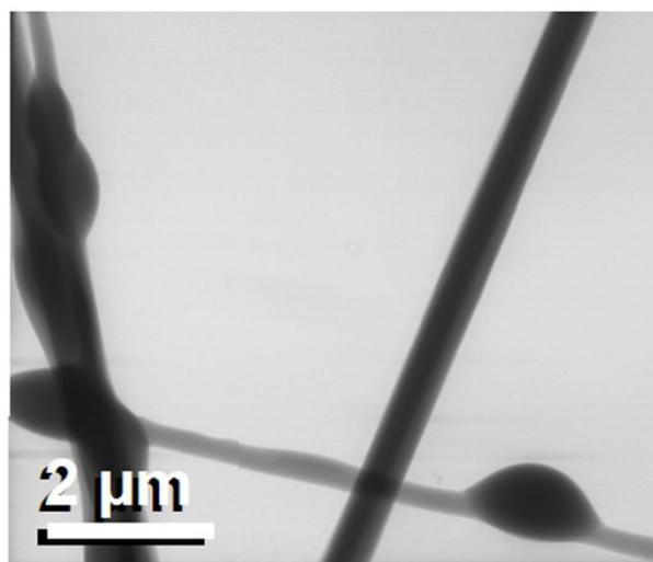
**Figure S5.** A TEM image of the products prepared from 8% w/v PVP and 30% w/v shellac solutions using the acentric spinneret II. The products generated are a combination of Janus fibers and particle-fiber structures consisting of shellac and PVP K60.
