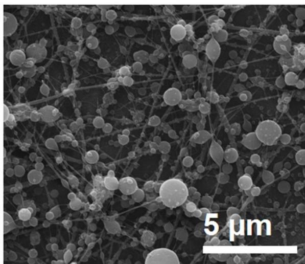
**Figure S2.** Preparation of nanofibers with 8% w/v PVP and 30% w/v shellac solutions using the parallel spinneret I. The products generated are observed to be a hybrid of PVP K60 nanofibers and shellac microparticles.
