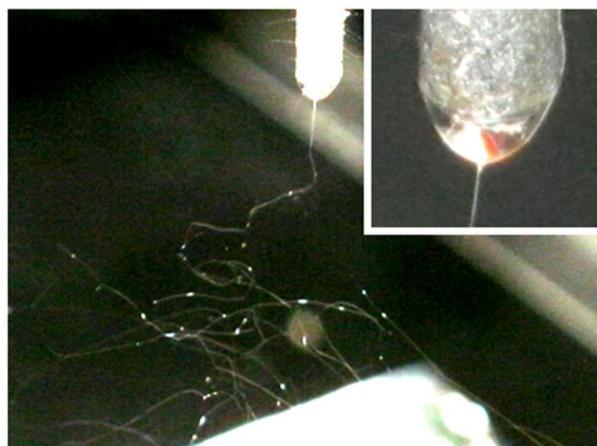
**Figure S3.** Preparation of nanofibers with 8% w/v PVP and 30% w/v shellac solutions using the acentric spinneret II. A stable Janus Taylor cone was observed, followed by bending and whipping.
