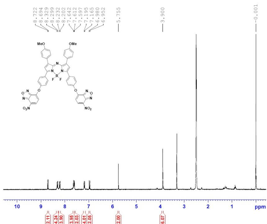
Fig. S26 <sup>1</sup>H NMR spectrum of compound 1.
