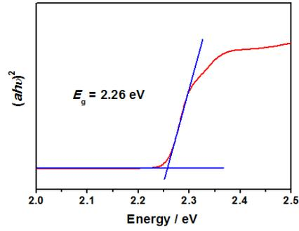
**Fig. S3.** Calculation of the optical bandgap (2.26 eV) *via* corresponding Tauc plots for the laminar MAPbBr<sub>3</sub> SC on TiO<sub>2</sub>-coated FTO glass.
