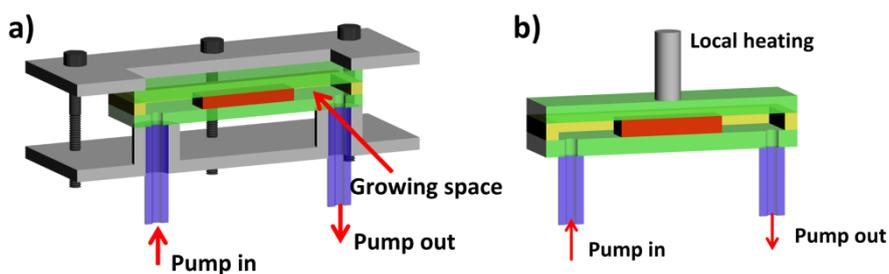
**Fig. S1.** Schematic diagram of growth module (a) and local heating with homothermal aluminium block (b) for the laminar  $\text{MAPbBr}_3$  SCs.
