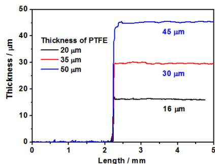
**Fig. S8.** Thickness curves of laminar MAPbBr<sub>3</sub> SCs with different PTFE thin membrane of 20, 35 and 50 μm *via* step profiler.
