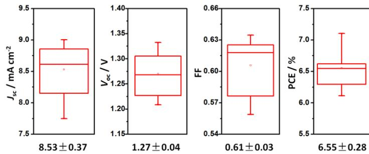
**Fig. S5.** The box-chart images of photovoltaic parameters for 20 devices which extracted from measuring *I-V* curves at simulated one sun illumination (100 mW cm<sup>-2</sup>, AM 1.5G).
