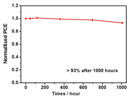
**Fig. S7.** The stability test of the cell (III) as a function of storage time in dry air without encapsulation.
