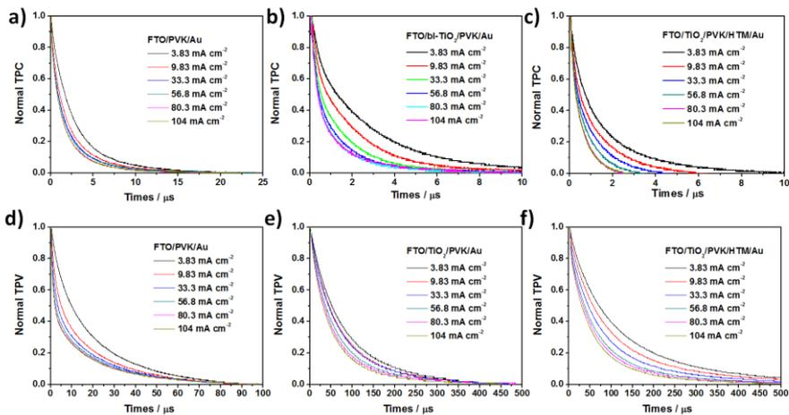
**Fig. S6.** TPC (a-c) and TPV (d-f) curves of cell (I) FTO/PVK/Au, (II) FTO/TiO<sub>2</sub>/PVK/Au and (III) FTO/TiO<sub>2</sub>/PVK/HTM/Au.
