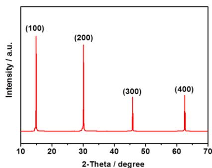
**Fig. S2.** XRD pattern of the flat  $\text{MAPbBr}_3$  SC on  $\text{TiO}_2$ -coated FTO glass.
