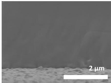
**Fig. S4.** High magnification SEM the interface of TiO<sub>2</sub> coated FTO glass/MAPbBr<sub>3</sub> SC.
