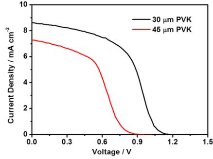
**Fig. S9.** The  $J$ - $V$  curves of cell (III) with 30 and 45  $\mu\text{m}$  thick  $\text{MAPbBr}_3$  SC at one sun illumination ( $100 \text{ mW cm}^{-2}$ , AM 1.5G).
