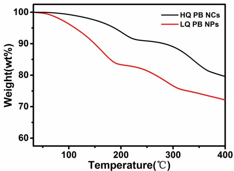
Figure S6. TG curves of the as-prepared HQ-PB NCs and LQ-PB NPs.
