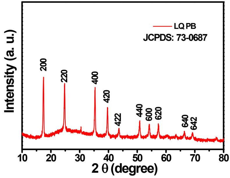
Fig. S1 The XRD pattern of the LQ-PB NPs.
