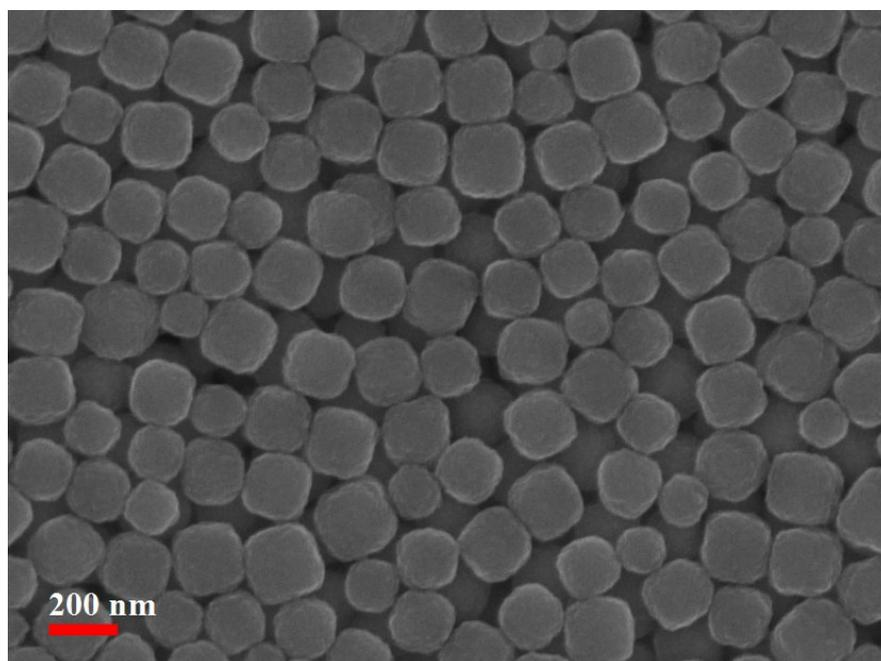
**Fig. S3** The SEM image of the LQ-PB NPs.
