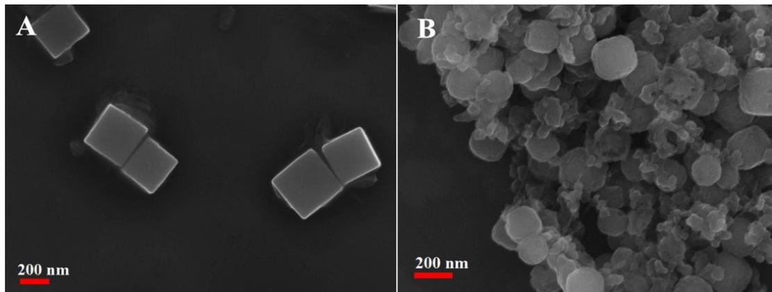
**Figure S8.** SEM images of the HQ-PB NCs and LQ-PB NPs after cycling test.
