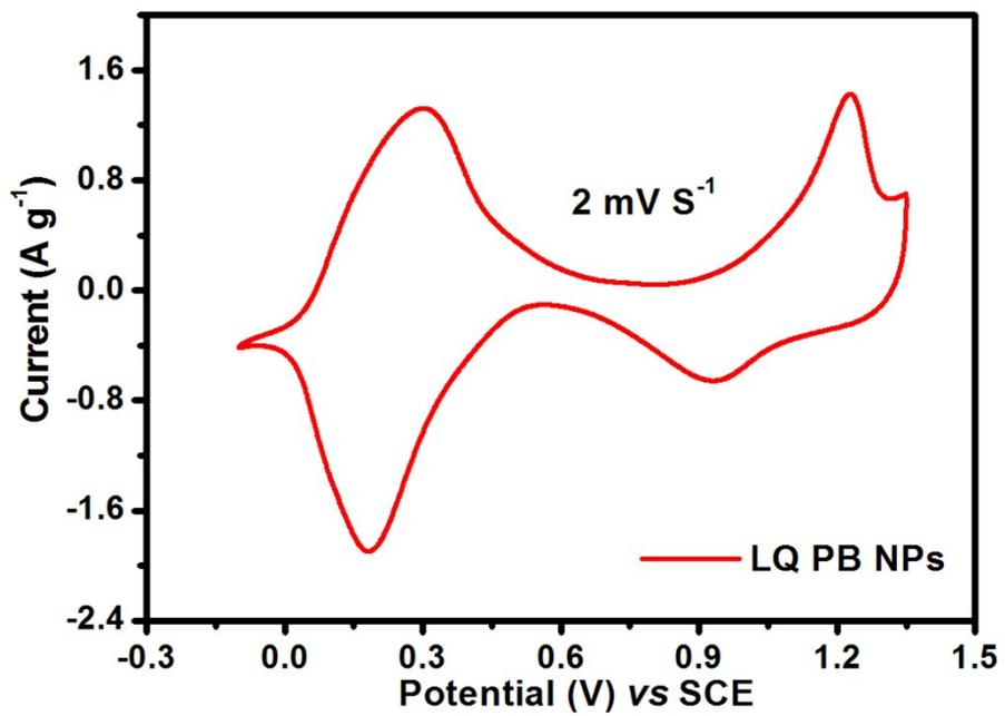
**Fig. S7** CV curve of the LQ-PB NPs recorded at a scan rate of 2 mV s<sup>-1</sup>.
