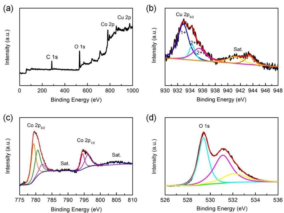
Fig. S4 XPS spectrums of  $\text{CuCo}_2\text{O}_4$ : (a) full spectrum, (b) Cu 2p spectrum, (c) Co 2p spectrum and (d) O 1s spectrum.
