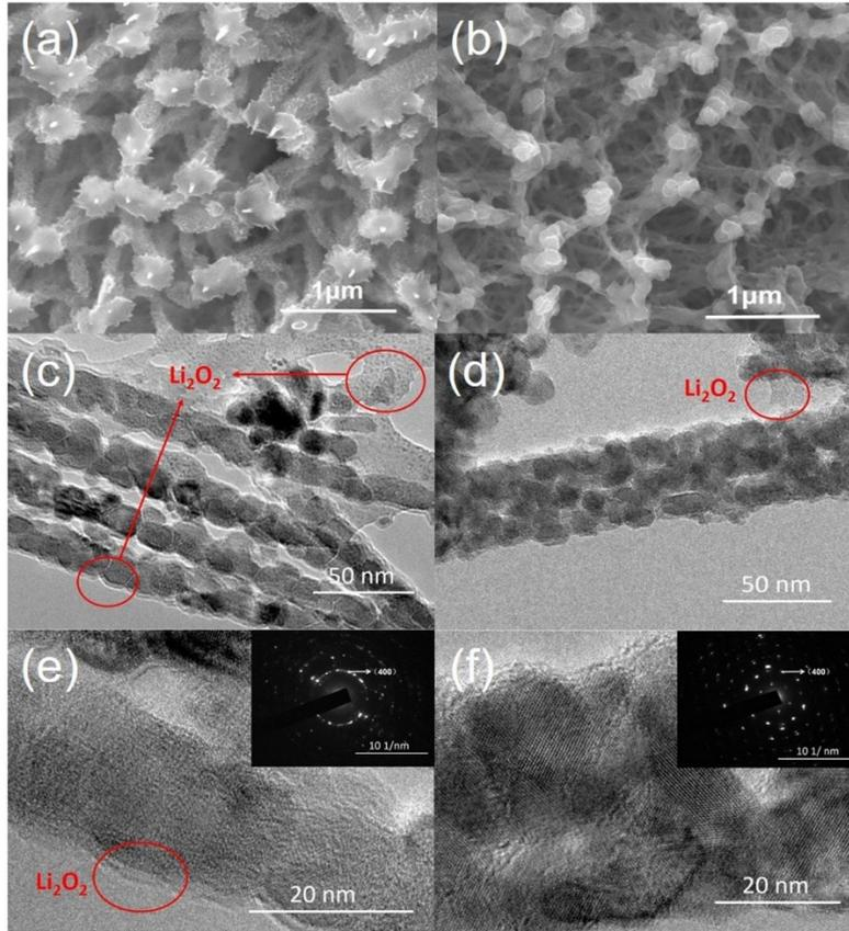
Fig. S6 SEM images of the electrode with CCO-Ni (a) after the first discharge and (b) after first charge; (c) TEM image of the electrode with CCO-Ni after the first discharge at  $0.1\text{mA cm}^{-2}$ , and the corresponding (e) HRTEM image and SAED pattern; (d) TEM image of the electrode with CCO-Ni after recharge at  $0.1\text{mA cm}^{-2}$ , and the corresponding (f) HRTEM image and SAED pattern.
