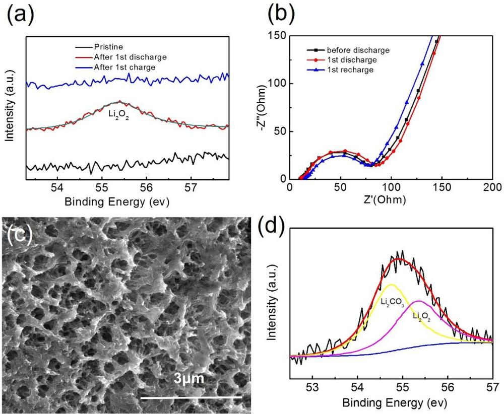
Fig. S7 XPS spectrum of Li 1s and (b) Nyquist plots of batteries with pristine electrode, after first discharge and after recharge; (c) SEM image of the electrode with CCO-Ni after 70 cycles; (d) the corresponding Li 1s XPS spectrum of the electrode with CCO-Ni after 70 cycles.
