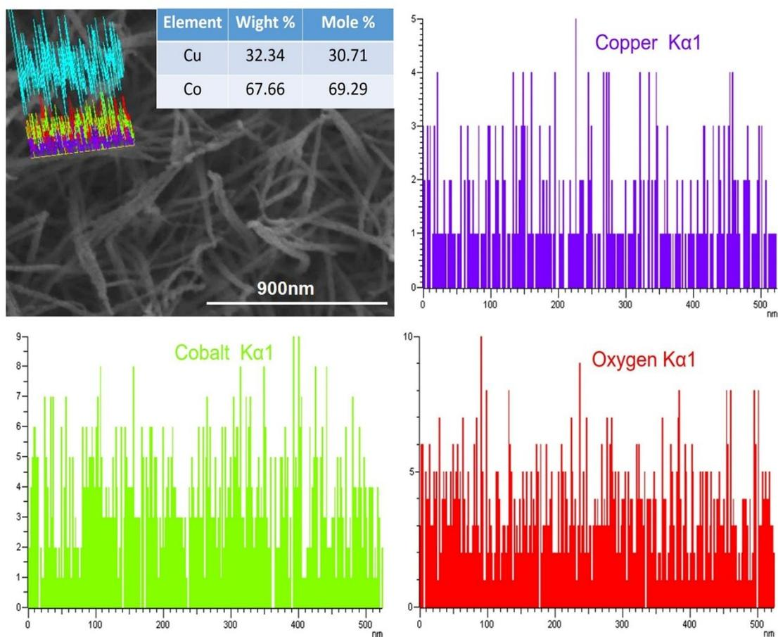
Fig. S3 EDS mapping images of the  $\text{CuCo}_2\text{O}_4$  nanowires on Ni foam.
