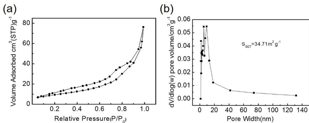
Fig. S2 (a) Nitrogen adsorption-desorption isotherms of CCO-Ni foam and (b) pore size distribution curves of CCO-Ni.
