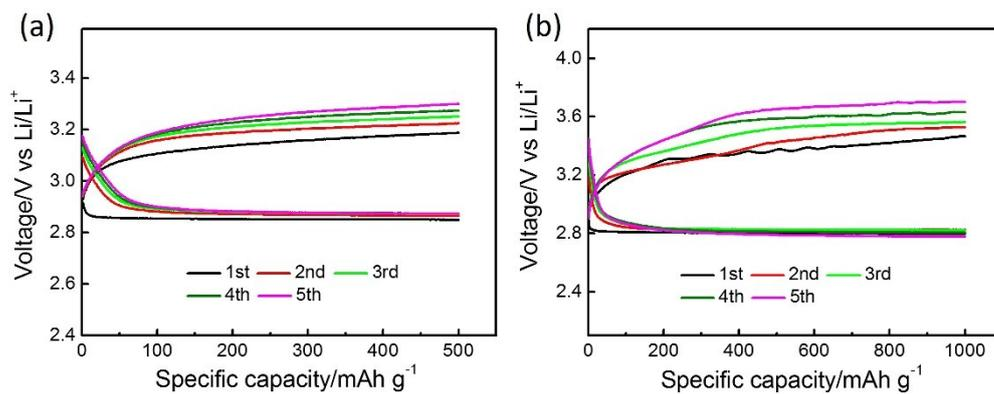
Fig.S5 Discharge-charge profiles of the initial five cycles of the Li-O<sub>2</sub> batteries with CCO-Ni cathodes at a current density of 0.1 mA cm<sup>-2</sup> with a cut-off capacity of (a) 500 mAh g<sup>-1</sup> and (b) 1000 mAh g<sup>-1</sup>.
