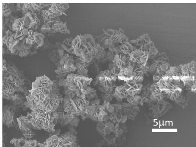
**Fig. S3** Scanning electron microscopy (SEM) images of the  $\text{CaCO}_3$  obtained by double-jet method at a rate of  $2 \text{ mL/h}$  at  $25 \text{ }^\circ\text{C}$  when the PEG-PNIPAM-PAMPS is absent, pure vaterite.  $[\text{CaCl}_2] = [\text{Na}_2\text{CO}_3] = 100 \text{ mM}$ . The injected solutions was added into  $10 \text{ mL}$  water in the reaction vessel for  $45 \text{ minutes}$ .
