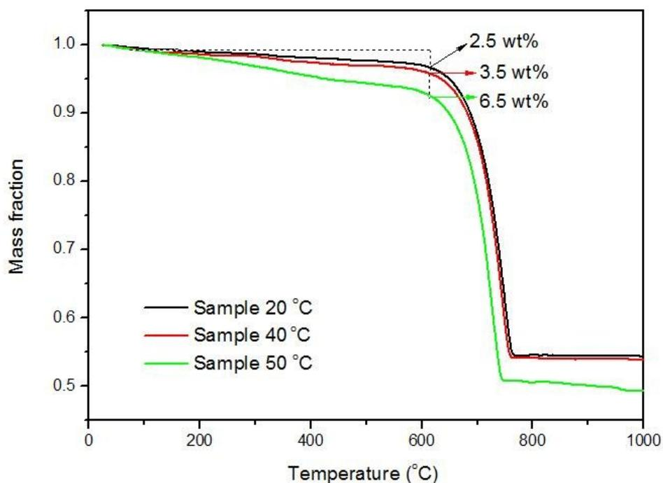
**Fig. S4** Thermogravimetric curves of the obtained CaCO<sub>3</sub> at different temperature
