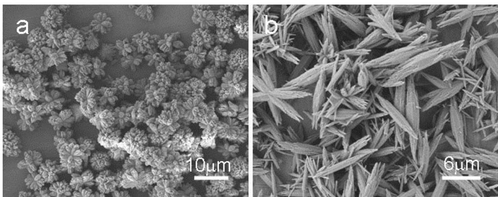
**Fig. S7** SEM images of the  $\text{CaCO}_3$  obtained by the double-jet method at a rate of  $2 \text{ ml/h}$  in presence of PEG-PNIPAM-PAMPS at  $50^\circ\text{C}$ . (a)  $[\text{polymer}] = 0.4 \text{ g L}^{-1}$ , volume =  $10 \text{ mL}$ , aragonite; (b)  $[\text{polymer}] = 0.05 \text{ g L}^{-1}$ , volume =  $10 \text{ mL}$ , aragonite.  $[\text{CaCl}_2] = 100 \text{ mM}$ , volume =  $1.5 \text{ mL}$ ;  $[\text{Na}_2\text{CO}_3] = 100 \text{ mM}$ , volume =  $1.5 \text{ mL}$ .
