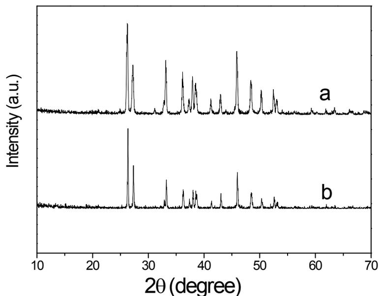
**Fig. S8** XRD patterns of the  $\text{CaCO}_3$  obtained by the double-jet method at a rate of 2 ml/h in presence of PEG-PNIPAM-PAMPS at  $50^\circ\text{C}$ : (a) [polymer] =  $0.4 \text{ g L}^{-1}$ , volume = 10 mL, aragonite; (b) [polymer] =  $0.05 \text{ g L}^{-1}$ , volume = 10 mL, aragonite.  $[\text{CaCl}_2] = 100 \text{ mM}$ , volume = 1.5 mL;  $[\text{Na}_2\text{CO}_3] = 100 \text{ mM}$ , volume = 1.5 mL.
