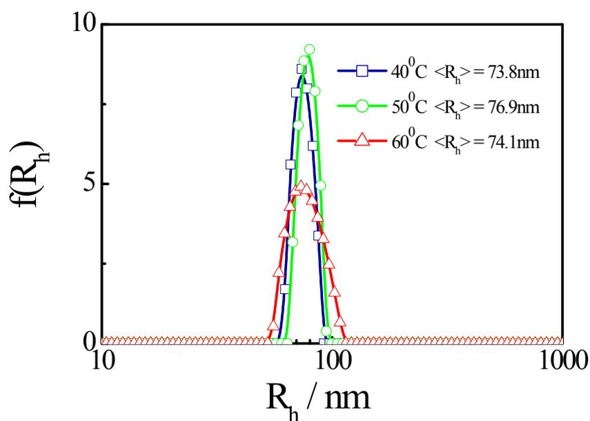
**Fig. S1** Distributions of hydrodynamic radius of the PEG-PNIPAM-PAMPS at 40°C, 50°C, 60°C.
