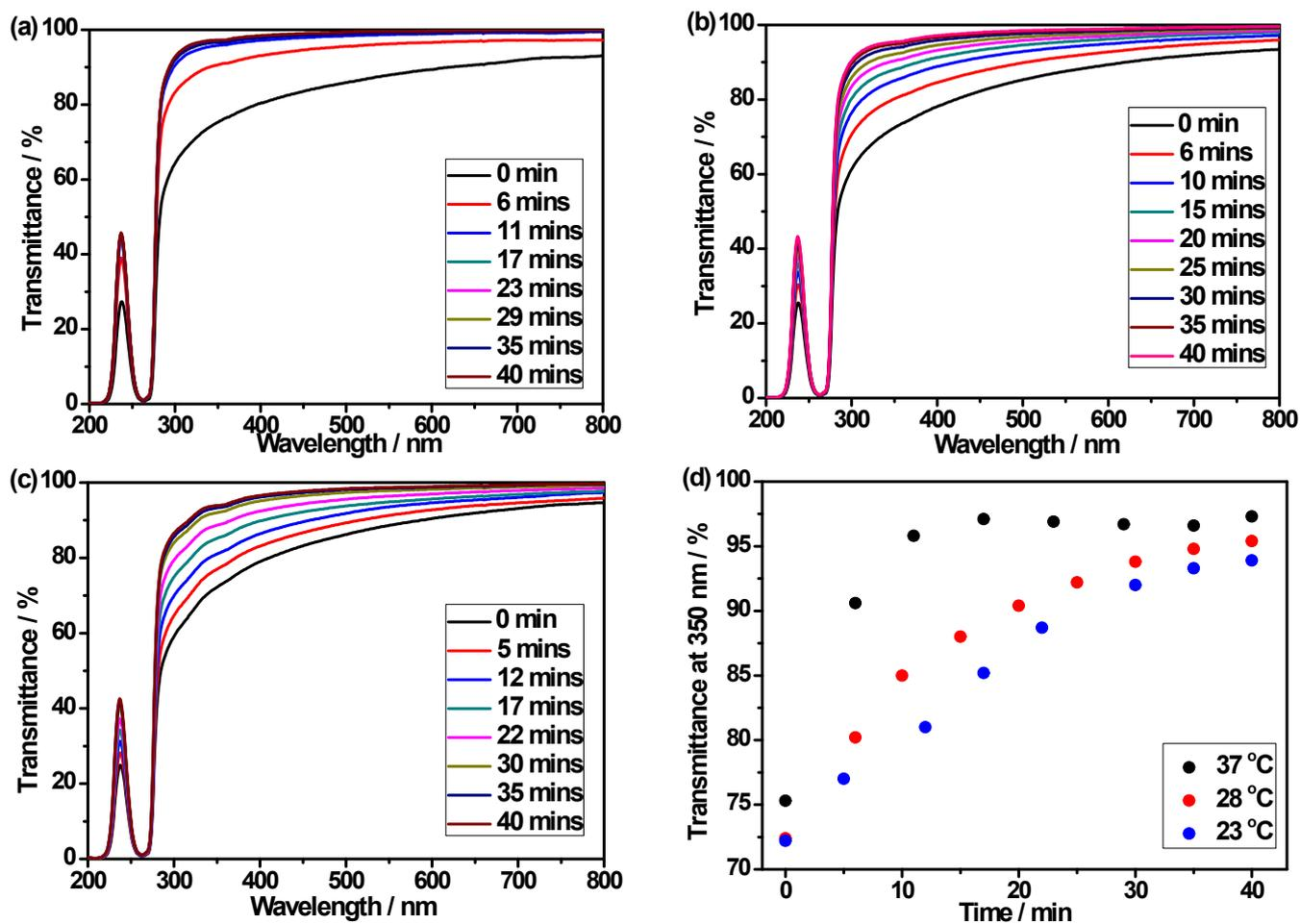
Fig. S18 Optical transmittance of the calixpyridinium-HA assembly at different time after addition of 10 U/mL HAase in water at 37 °C (a), 28 °C (b) and 23 °C (c). (d) Dependence of the optical transmittance of the calixpyridinium-HA solution at 350 nm on time in the presence of 10 U/mL HAase at different temperatures in water. [calixpyridinium] = 0.10 mM, and [HA] = 1.40  $\mu$ M.
