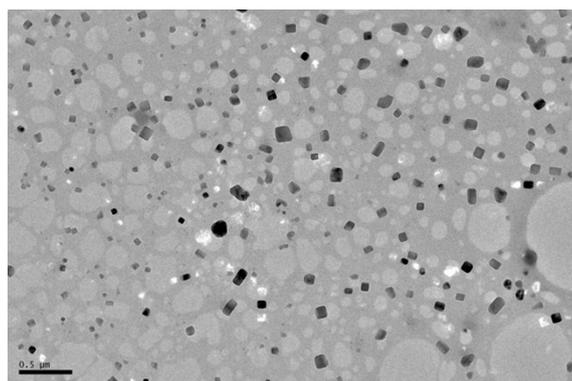
**Fig. S24** High-resolution TEM image of the calixpyridinium–HA assembly prepared at 60 °C, [calixpyridinium] = 0.10 mM, and [HA] = 1.40  $\mu$ M.
