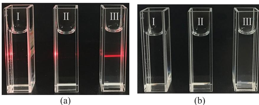
Fig. S3 Photos showing the Tyndall effect (a) and turbidity (b) of free calixpyridinium (I), free HA (II), and calixpyridinium-HA complex (III) in water, [calixpyridinium] = 0.10 mM, and [HA] = 1.40  $\mu\text{M}$ .
