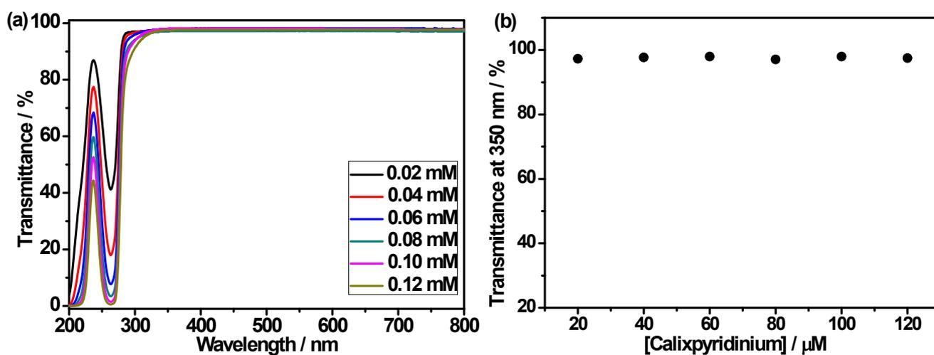
Fig. S7 (a) Optical transmittance of aqueous solutions of calixpyridinium at different concentrations from 20 to 120  $\mu\text{M}$  at room temperature. (b) Dependence of the optical transmittance at 350 nm on calixpyridinium concentration.
