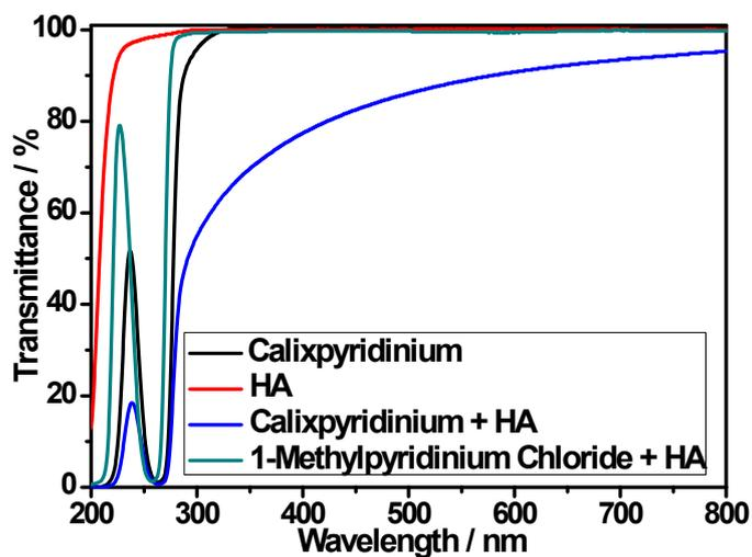
Fig. S9 Optical transmittance of calixpyridinium, HA, calixpyridinium+HA, and 1-methylpyridinium+HA at room temperature in water, [calixpyridinium] = 0.10 mM, [HA] = 1.40  $\mu$ M, and [1-methylpyridinium chloride] = 0.45 mM.
