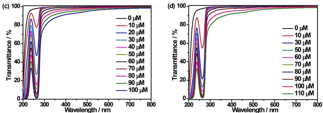
Fig. S4 Optical transmittance of aqueous solutions of calixpyridinium at different concentrations in the presence of 0.52  $\mu\text{M}$  (a), 0.78  $\mu\text{M}$  (b), 0.99  $\mu\text{M}$  (c), and 1.56  $\mu\text{M}$  (d) HA.
