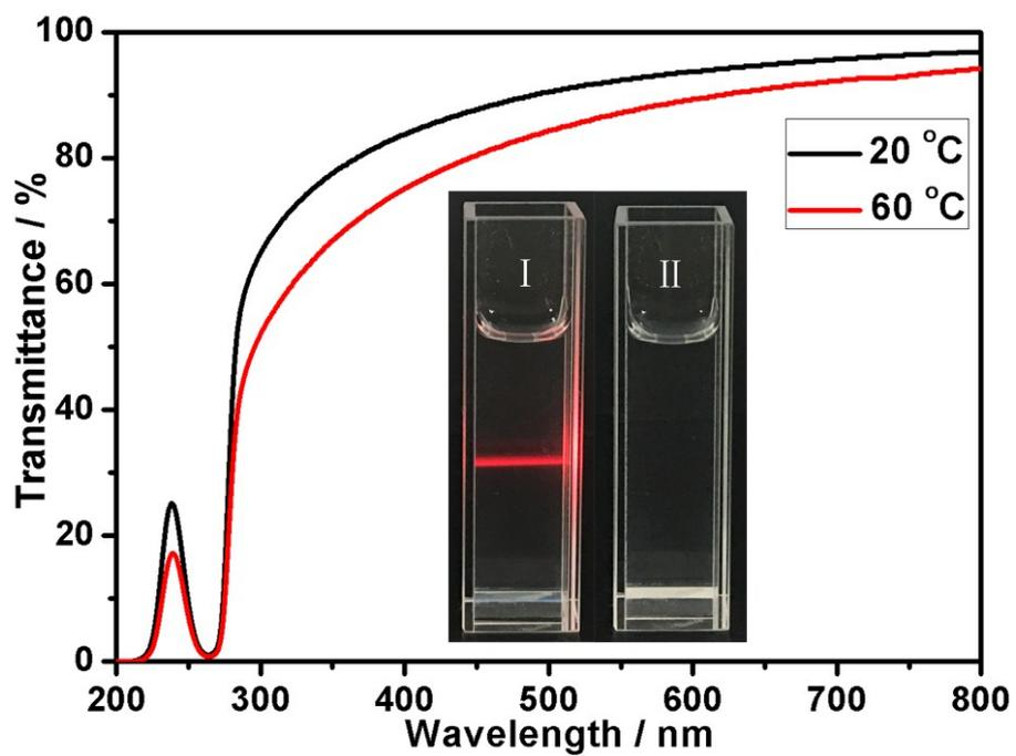
**Fig. S23** Optical transmittance of the calixpyridinium–HA assembly at 20 and 60 °C in water. Inset: photos showing the Tyndall effect (I) and turbidity (II) of the calixpyridinium–HA assembly at 60 °C in water. [calixpyridinium] = 0.10 mM, and [HA] = 1.40  $\mu$ M.
