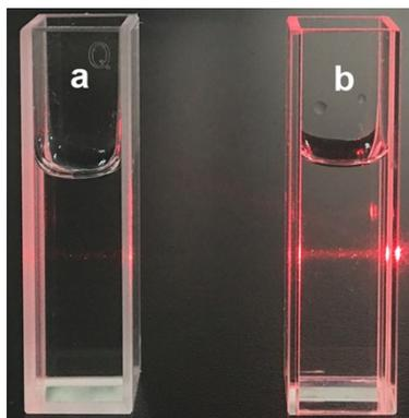
Fig. S2 Photos showing the Tyndall effect of free HA at different concentrations, [HA] = 78  $\mu\text{M}$  (a) and [HA] = 156  $\mu\text{M}$  (b).
