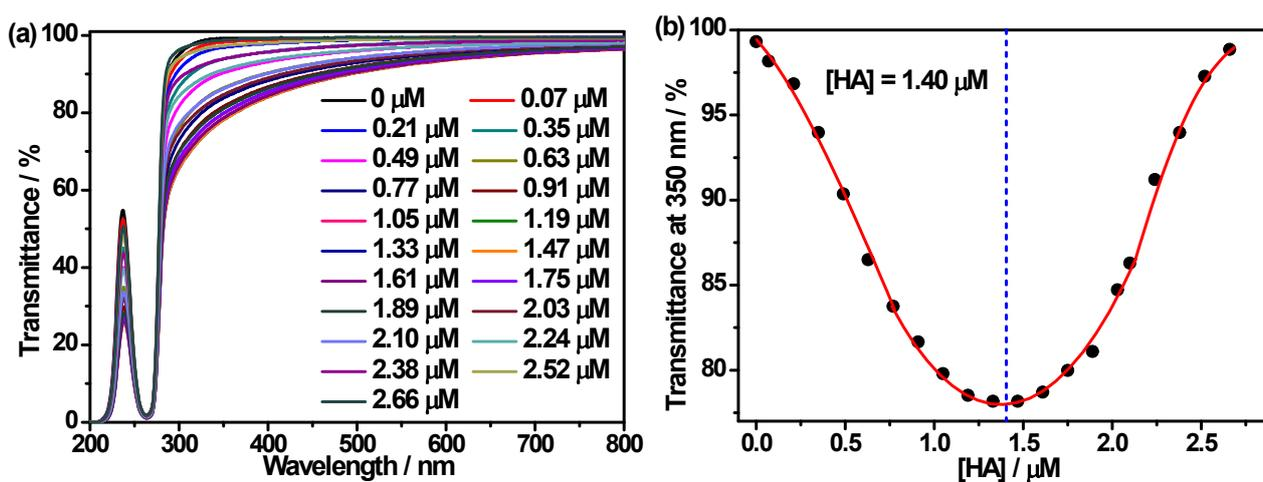
Fig. S8 (a) Optical transmittance of calixpyridinium (0.10 mM) by increasing the concentration of HA from 0 to 2.66  $\mu\text{M}$  at room temperature in water. (b) Dependence of the optical transmittance at 350 nm on the HA concentration with a fixed calixpyridinium concentration of 0.10 mM.
