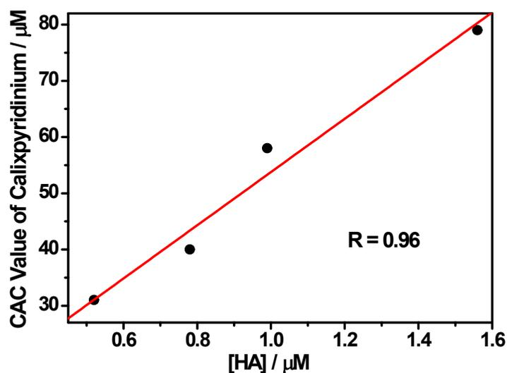
Fig. S6 Linear relationship between the CAC values of calixpyridinium and the concentrations of HA in water.
