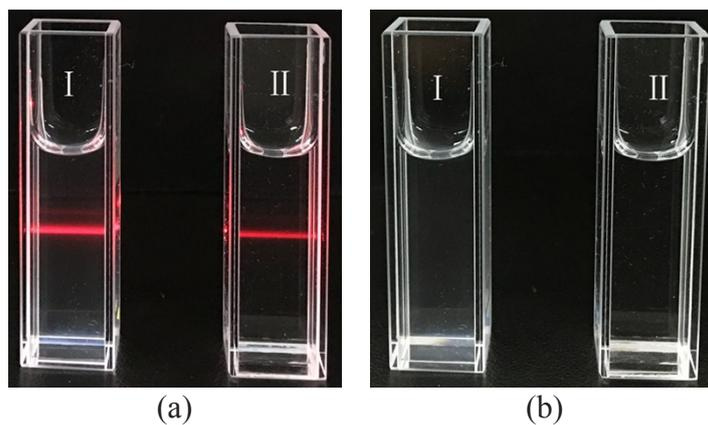
**Fig. S15** Photos showing the Tyndall effect (a) and turbidity (b) of the calixpyridinium–HA assembly before (I) and after addition of HAase for 30 minutes (II), [calixpyridinium] = 0.10 mM, [HA] = 1.40  $\mu$ M, and [HAase] = 10 U/mL.
