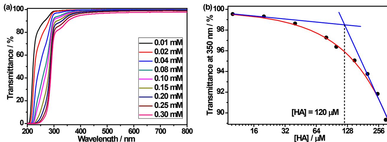
Fig. S1 (a) Optical transmittance of aqueous solutions of HA at different concentrations from 0.01 to 0.30 mM at room temperature. (b) Dependence of the optical transmittance at 350 nm on HA concentration.
