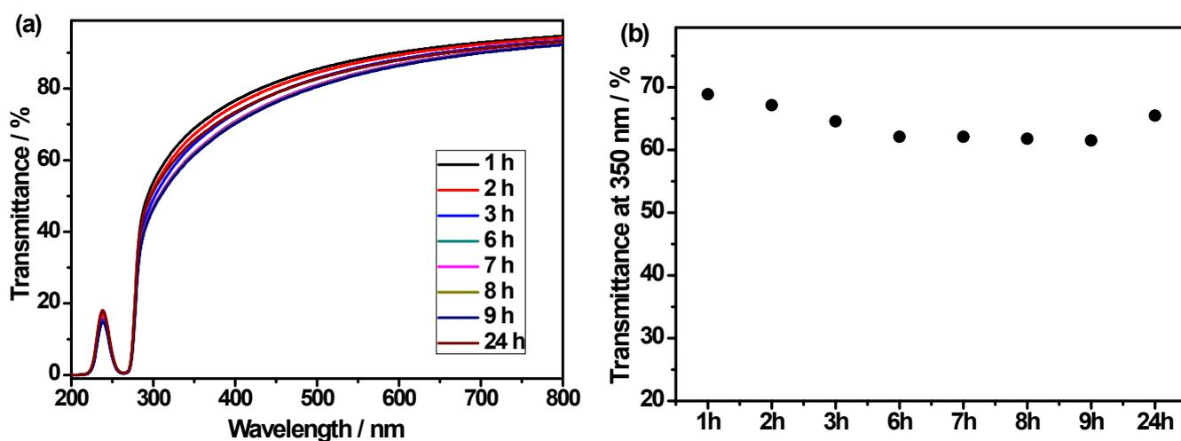
**Fig. S22** (a) Optical transmittance of the calixpyridinium-HA assembly at different time within 24 h at room temperature in water. (b) Dependence of the optical transmittance at 350 nm on time. [calixpyridinium] = 0.10 mM, and [HA] = 1.40  $\mu$ M.
