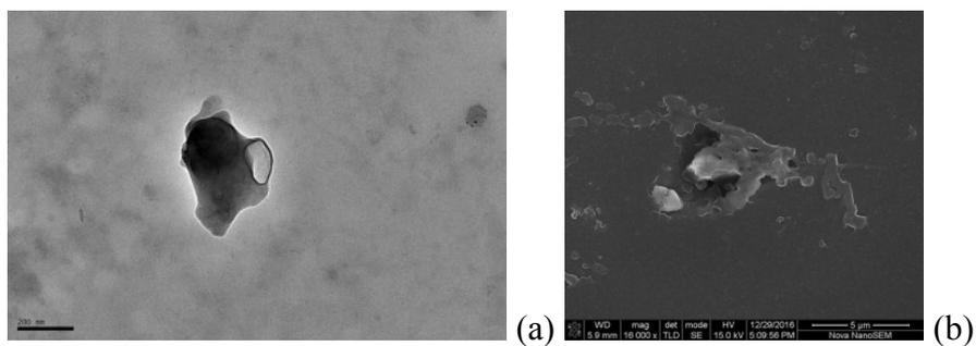
**Fig. S17** High-resolution TEM (a) and SEM (b) images of the calixpyridinium–HA assembly after addition of 10 U/mL HAase for 30 minutes.
