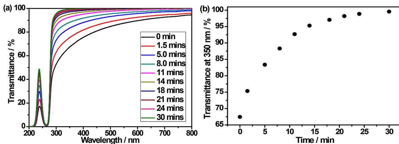
Fig. S14 (a) Optical transmittance of the calixpyridinium-HA assembly at different time after addition of 3 U/mL HAase in water at 37 °C. (b) Dependence of the optical transmittance of the calixpyridinium-HA solution at 350 nm on time in the presence of 3 U/mL HAase. [calixpyridinium] = 0.10 mM, and [HA] = 1.40  $\mu$ M.
