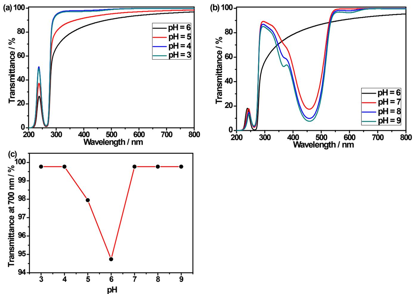
Fig. S10 (a and b) Optical transmittance of the aqueous solutions of the calixpyridinium-HA assembly at different pH values, [calixpyridinium] = 0.10 mM, and [HA] = 1.40  $\mu$ M. (c) Dependence of the optical transmittance at 700 nm on the pH values of the calixpyridinium-HA aqueous solutions.
