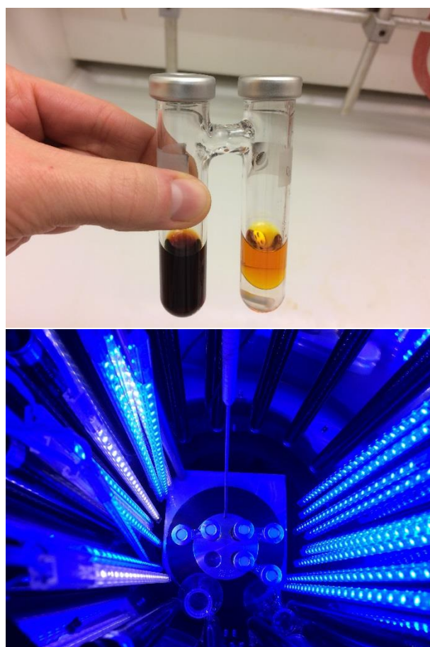
Figure S1. a) Double-chamber system, \text{C}_{\text{CO}} is the left chamber and \text{C}_{\text{rxn}} is the right chamber. b) Experimental set-up.
