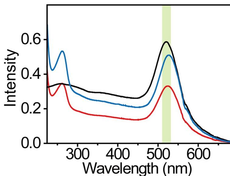
Fig. S2 UV-Vis spectra of AuNP (black), recognition sequences/AuNP (blue), and recognition sequences/nanoflares/AuNP (red).
