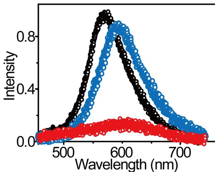
Fig. S6 The scattering spectra of AuNP (black), recognition sequences/AuNP (blue), and recognition sequences/nanoflares/AuNP (red).
